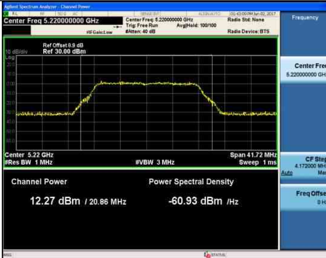
Maximum Conduct Output Power_11A_5240_Ant2
