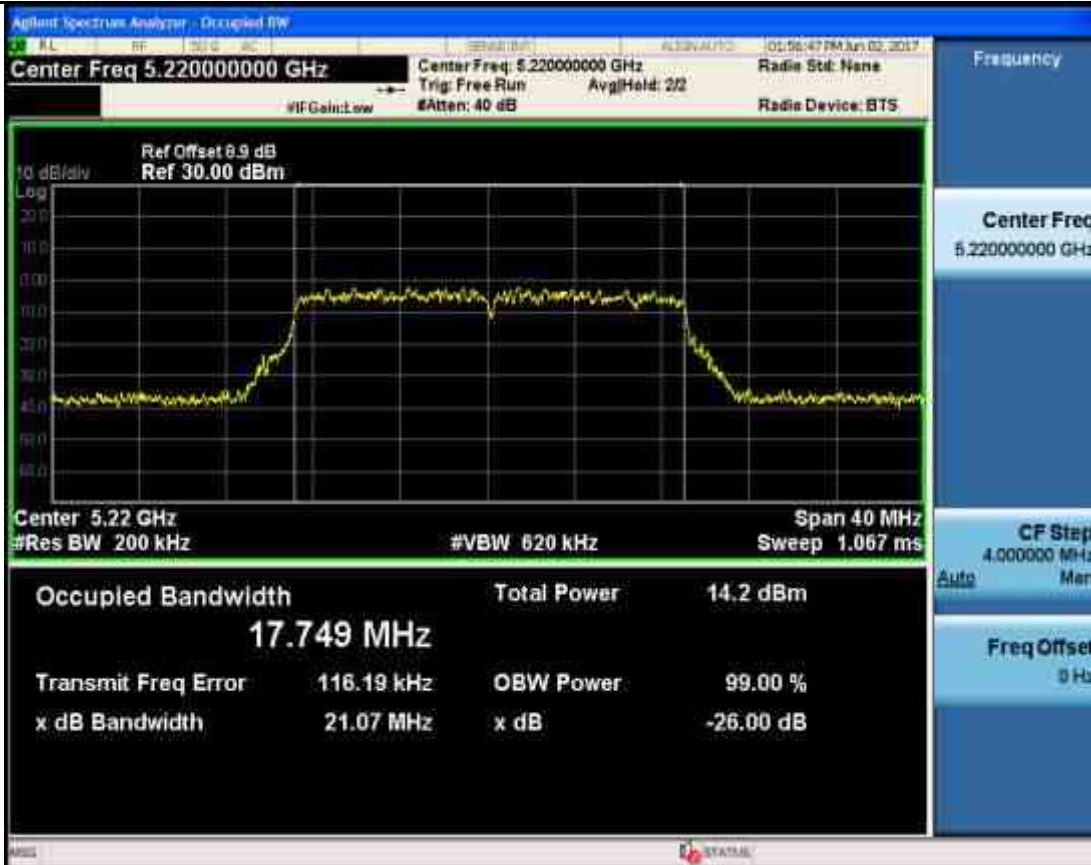
Occupied Bandwidth Measurement_11N20_5240_Ant2
