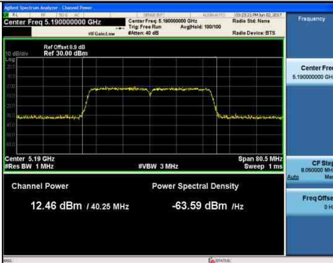
Maximum Conduct Output Power_11N40_5230_Ant2
