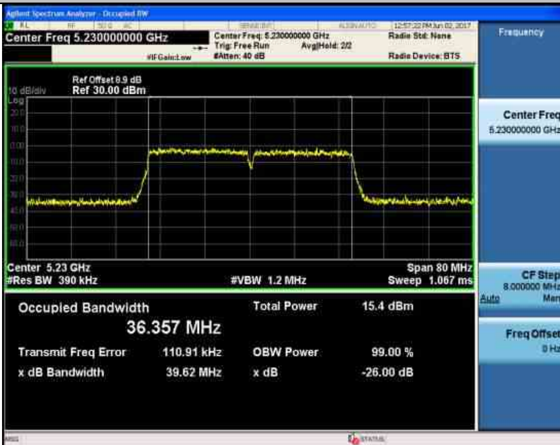
Occupied Bandwidth Measurement_11N40_5755_Ant1
