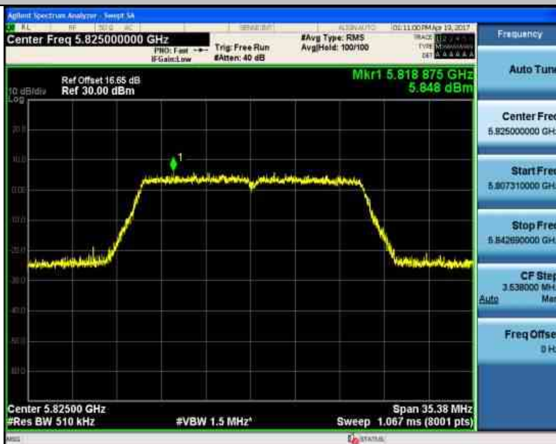
Maximum Conduct Output Power_TNVN_11N40_5190_Ant2
