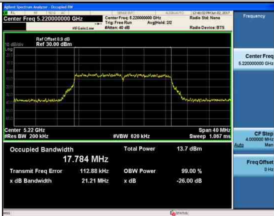
Emission Bandwidth Measurement_11N20_5240_Ant1
