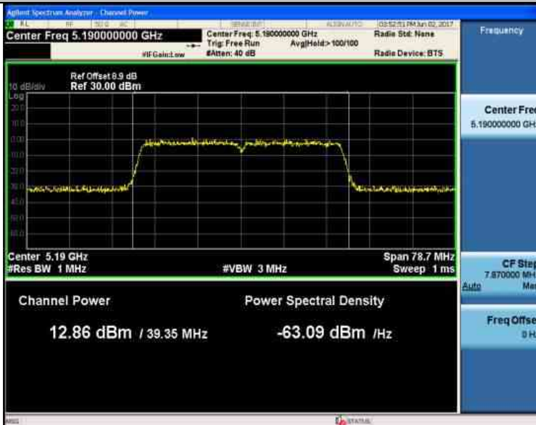
Maximum Conduct Output Power_11AC40_5230_Ant2
