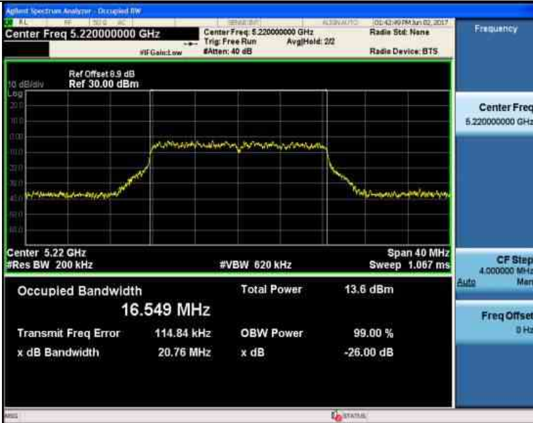
Occupied Bandwidth Measurement_11A_5240_Ant2
