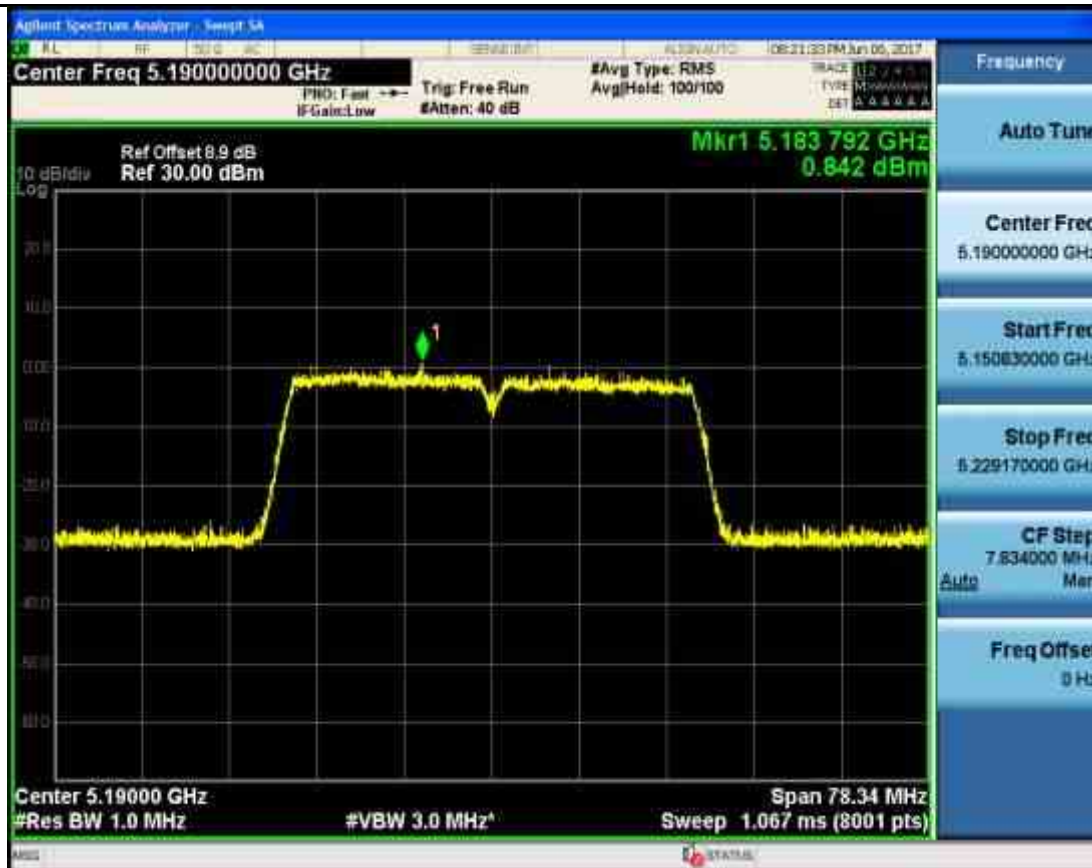
Maximum Conduct Output Power_TNVN_11AC40_5230_Ant2
