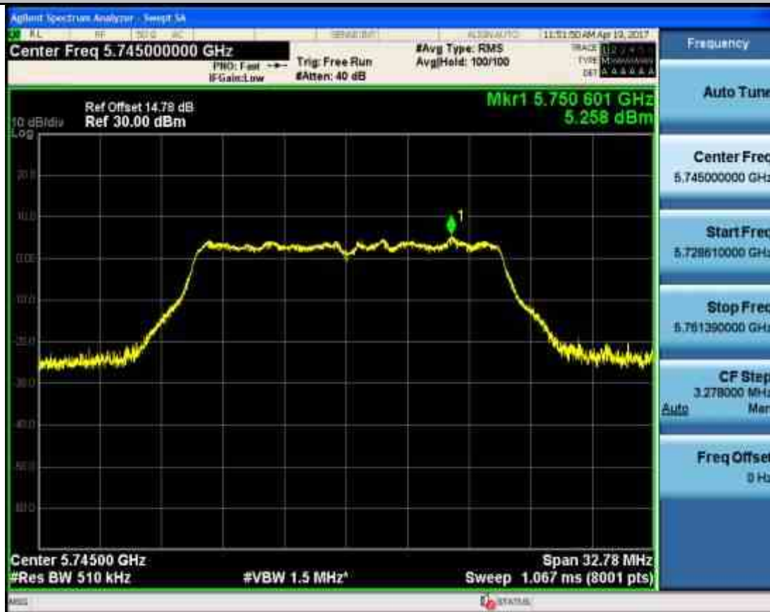
Maximum Conduct Output Power_TNVN_11A_5785_Ant2
