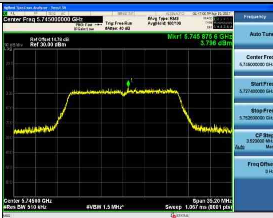
Maximum Conduct Output Power_TNVN_11AC20_5785_Ant2
