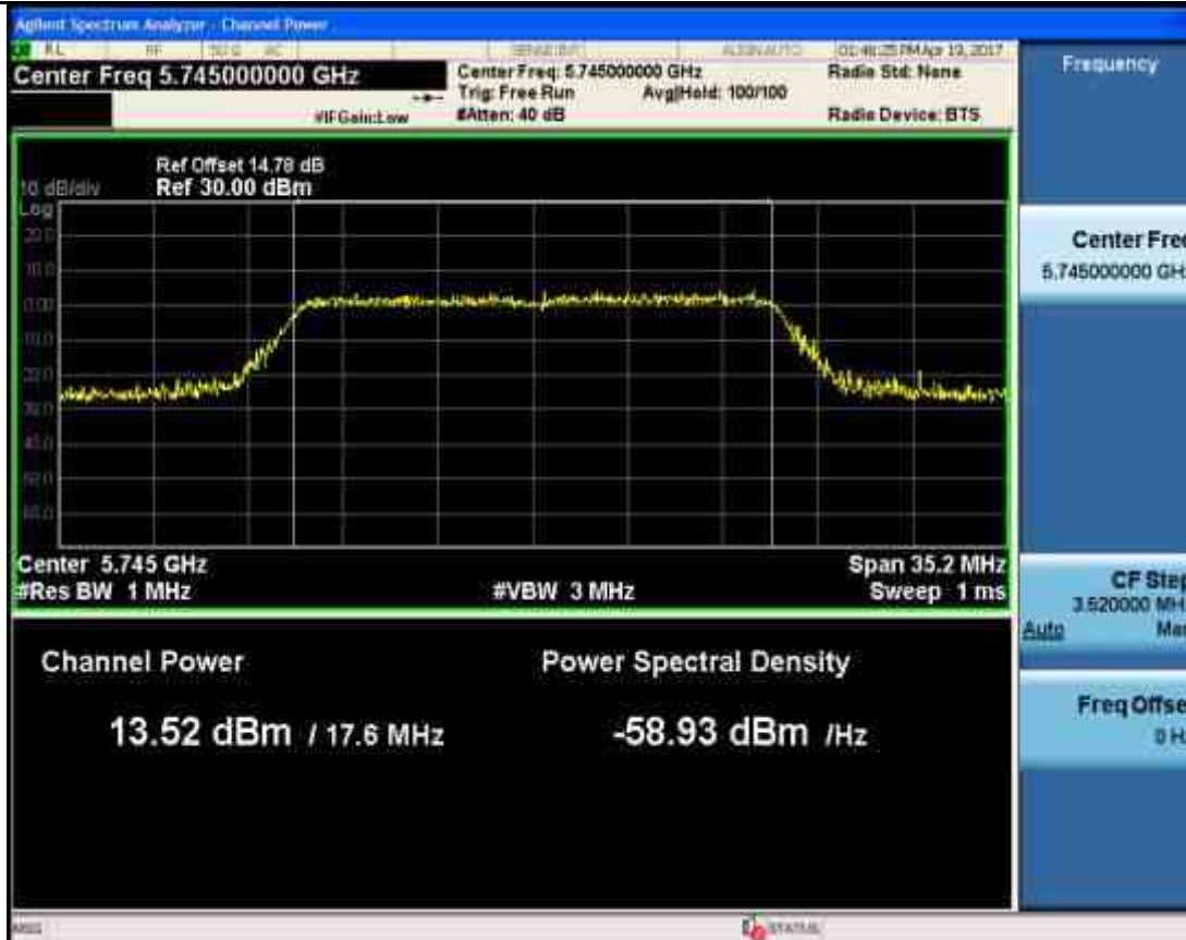
Maximum Conduct Output Power_11AC20_5785_Ant2
