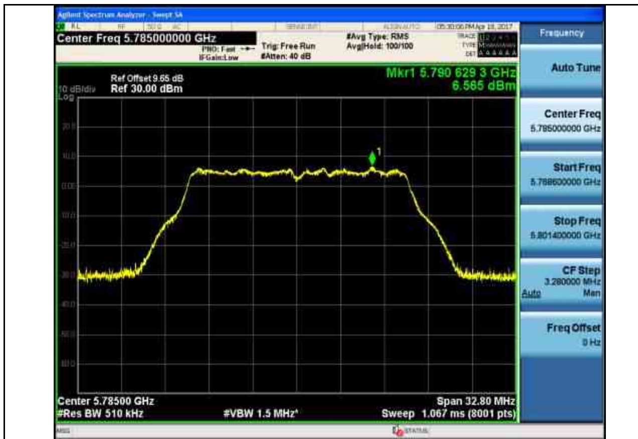
Maximum Conduct Output Power_TNVN_11A_5825_Ant1
