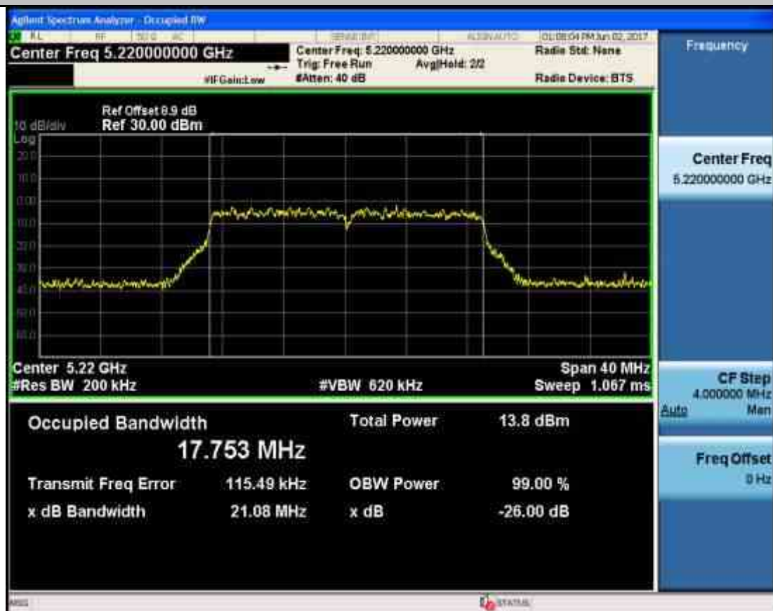
Emission Bandwidth Measurement_11AC20_5240_Ant1
