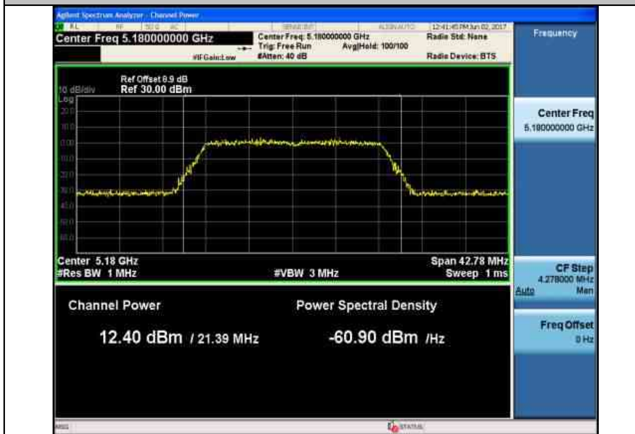
Maximum Conduct Output Power_11N20_5220_Ant1
