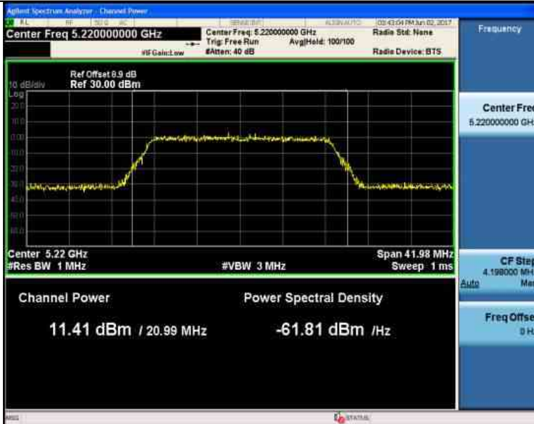
Maximum Conduct Output Power_11AC20_5240_Ant2
