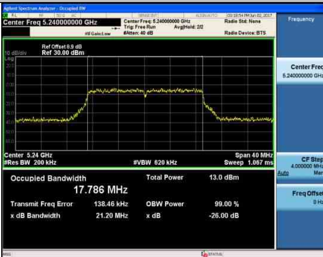
Occupied Bandwidth Measurement_11N20_5745_Ant2
