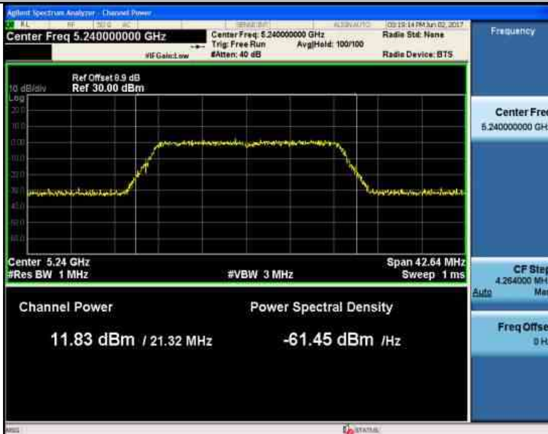
Maximum Conduct Output Power_11N20_5745_Ant2
