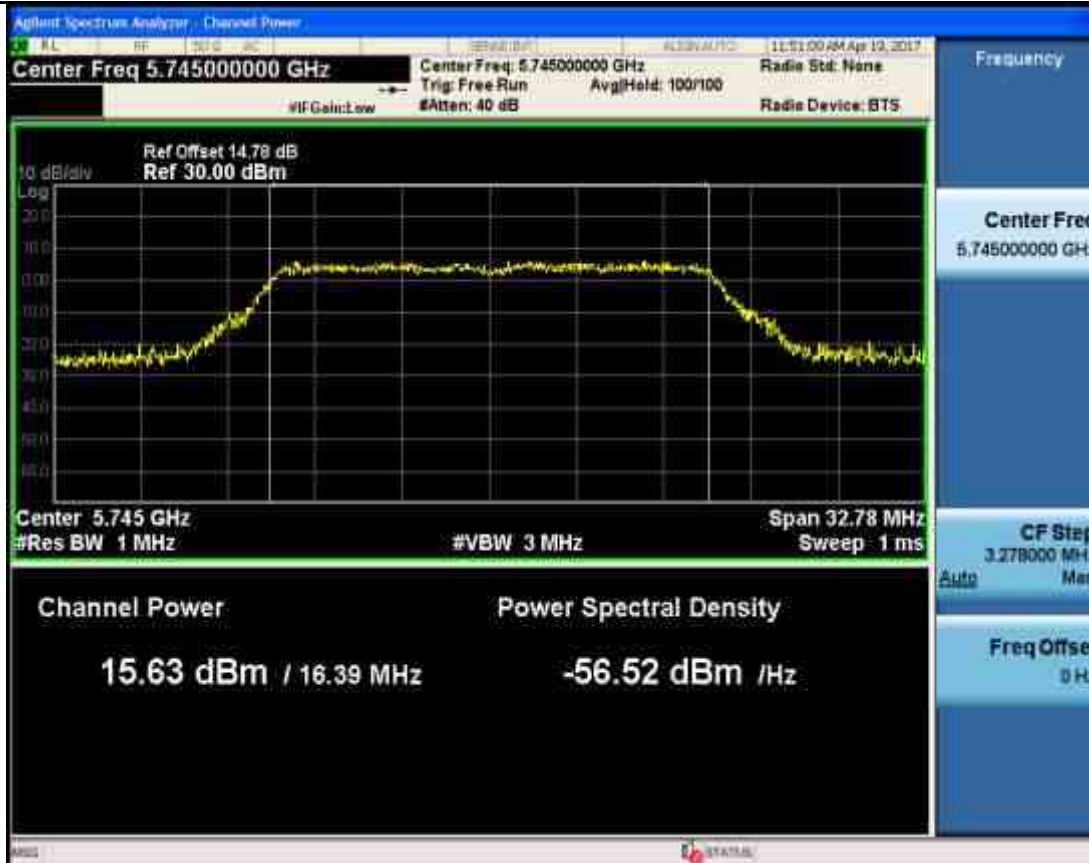
Maximum Conduct Output Power_11A_5785_Ant2
