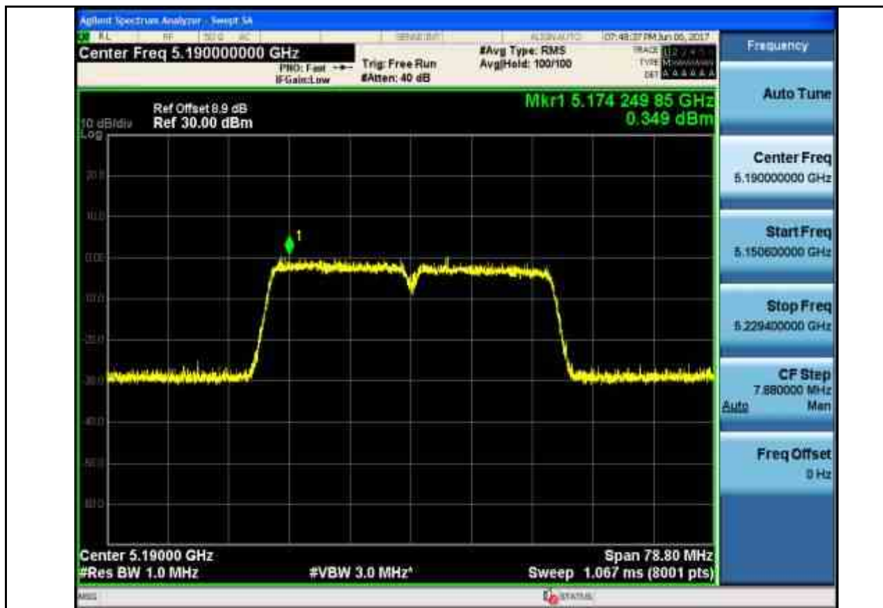
Maximum Conduct Output Power_TNVN_11AC40_5230_Ant1
