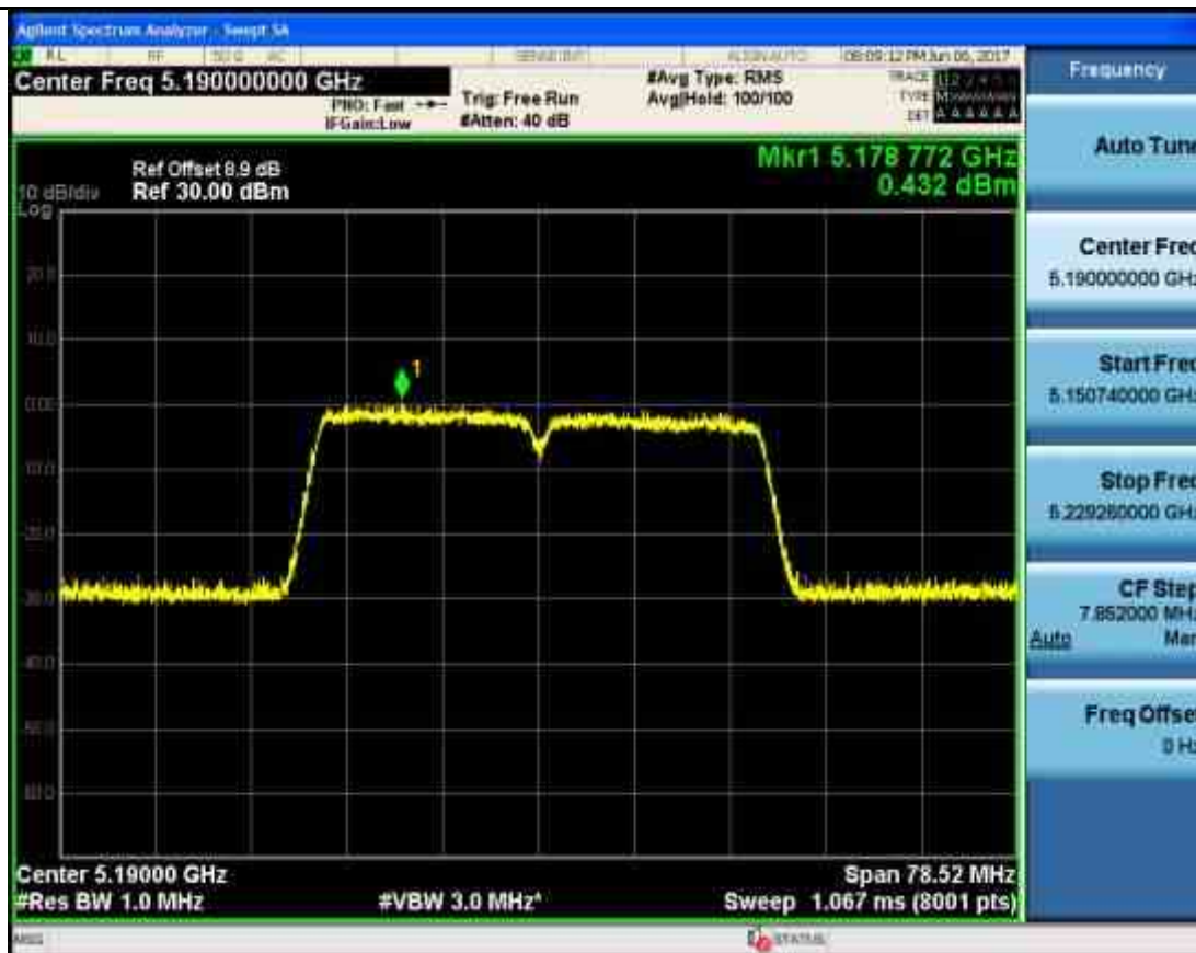
Maximum Conduct Output Power_TNVN_11N40_5230_Ant2
