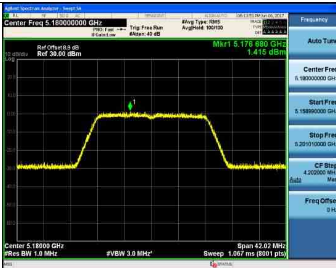
Maximum Conduct Output Power_TNVN_11AC20_5220_Ant2
