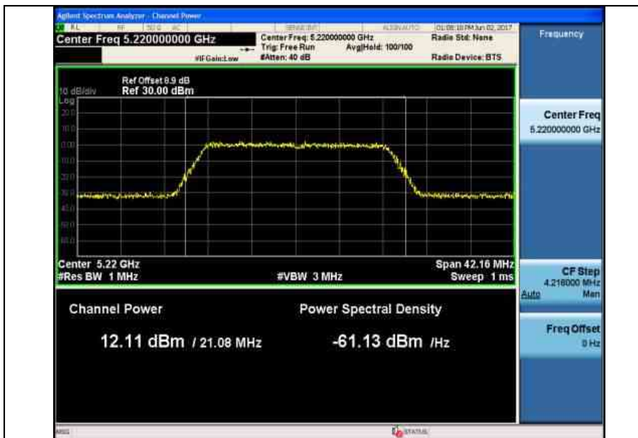
Maximum Conduct Output Power_11AC20_5240_Ant1
