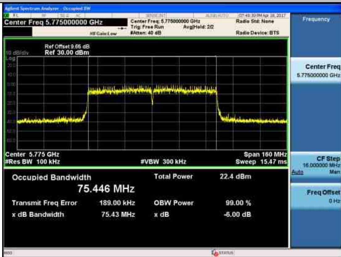
Emission Bandwidth Measurement_11AC80_5775_Ant1
