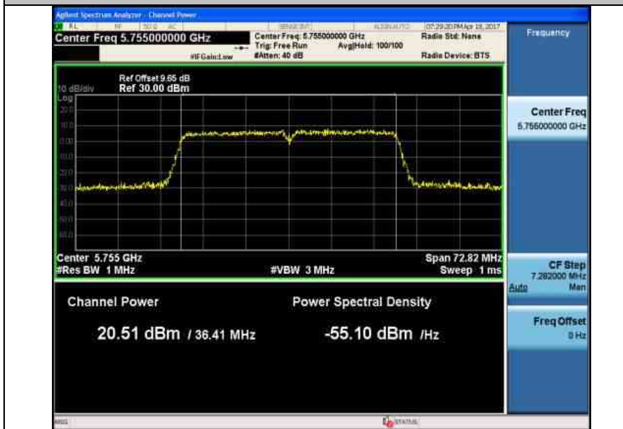
Maximum Conduct Output Power_11AC40_5795_Ant1
