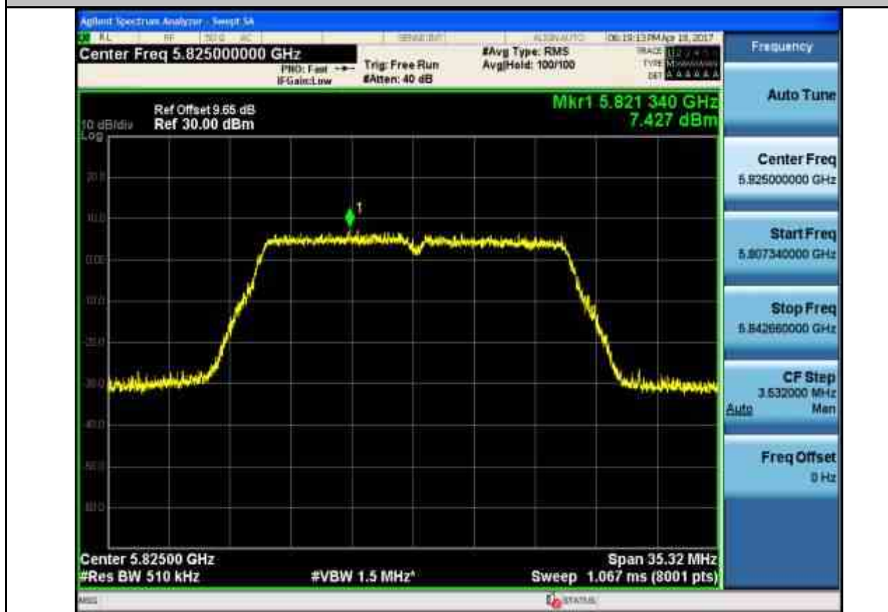
Maximum Conduct Output Power_TNVN_11N40_5190_Ant1
