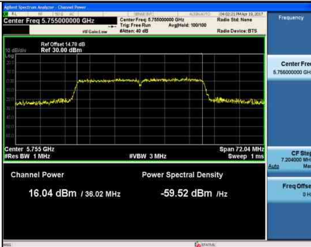
Maximum Conduct Output Power_11AC40_5795_Ant2
