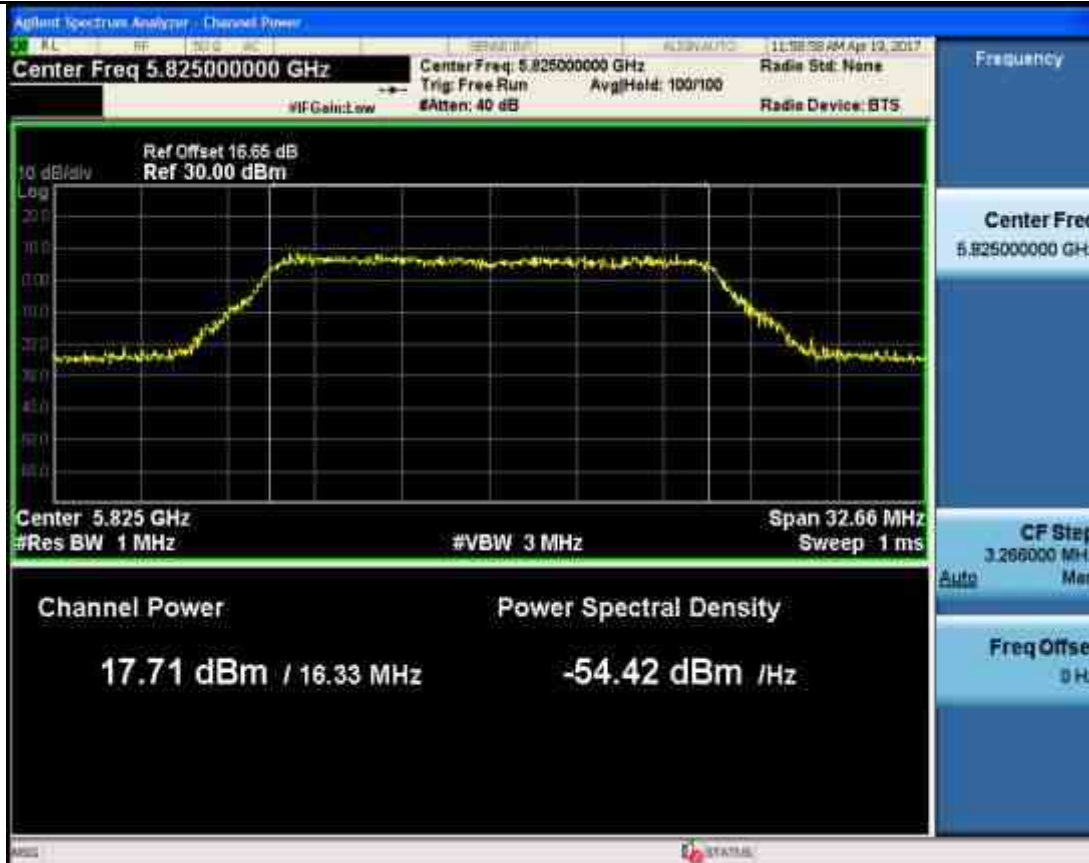
Maximum Conduct Output Power_11N20_5180_Ant2
