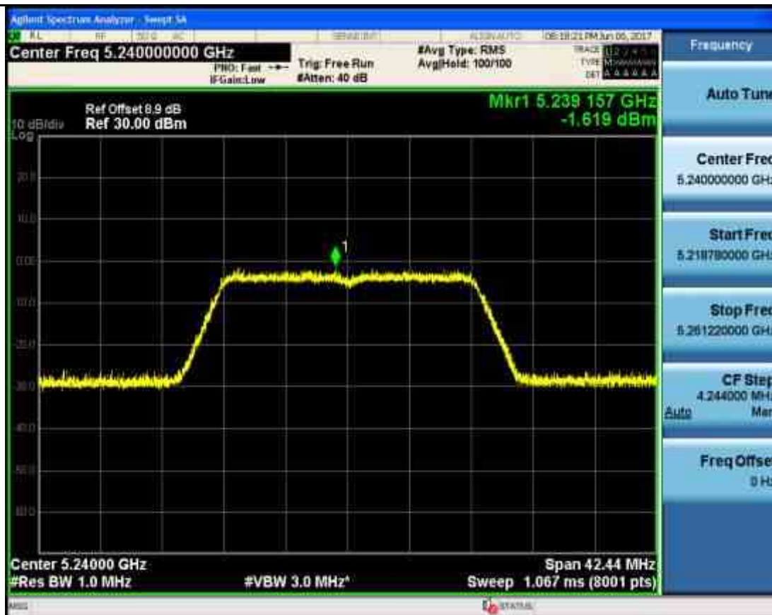
Maximum Conduct Output Power_TNVN_11AC20_5745_Ant2
