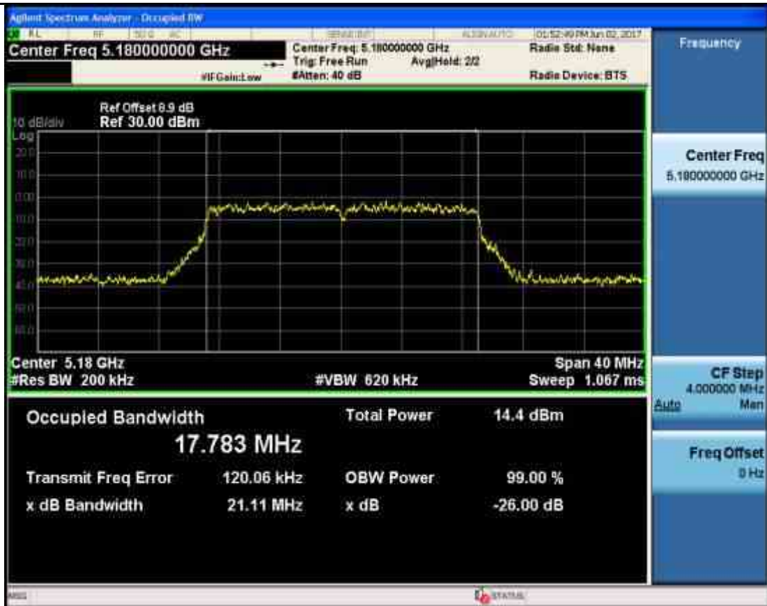
Emission Bandwidth Measurement_11N20_5220_Ant2
