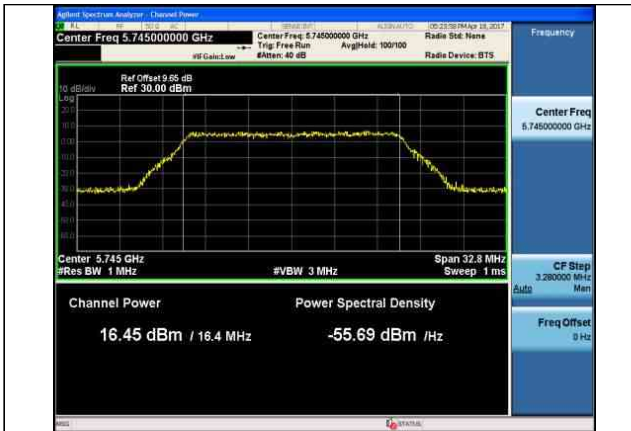
Maximum Conduct Output Power_11A_5785_Ant1
