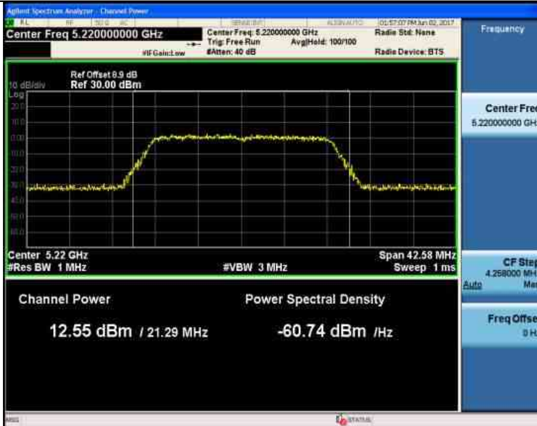
Maximum Conduct Output Power_11N20_5240_Ant2
