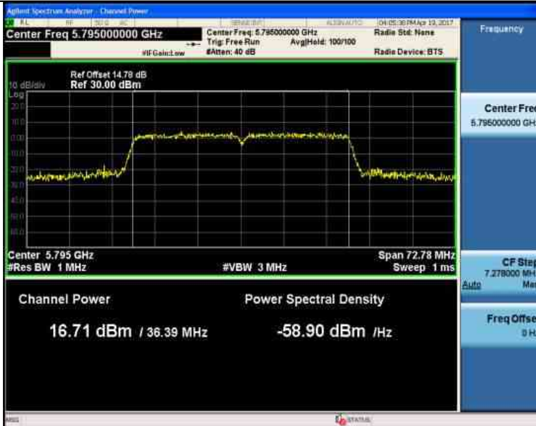
Maximum Conduct Output Power_11AC80_5210_Ant2
