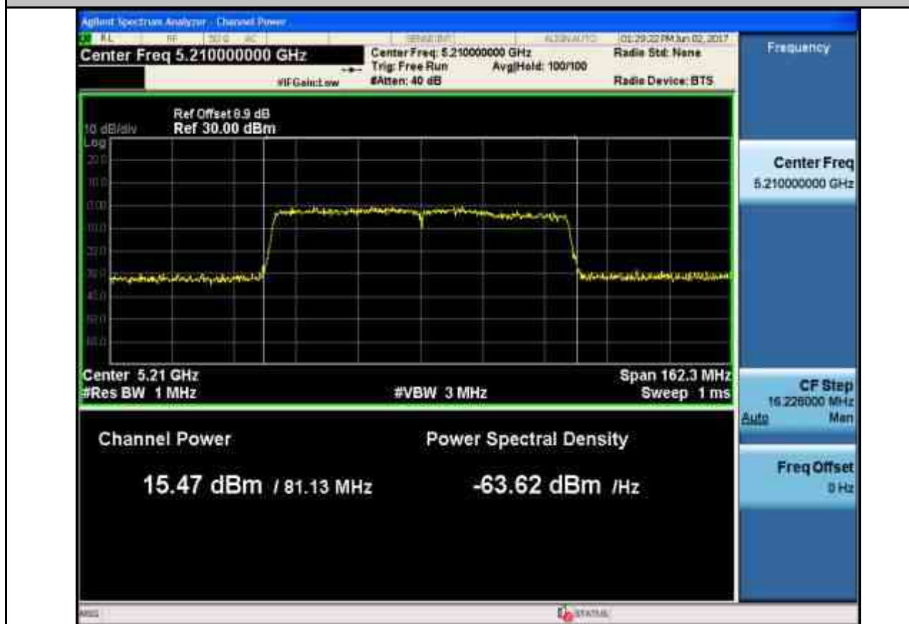
Maximum Conduct Output Power_11AC80_5775_Ant1
