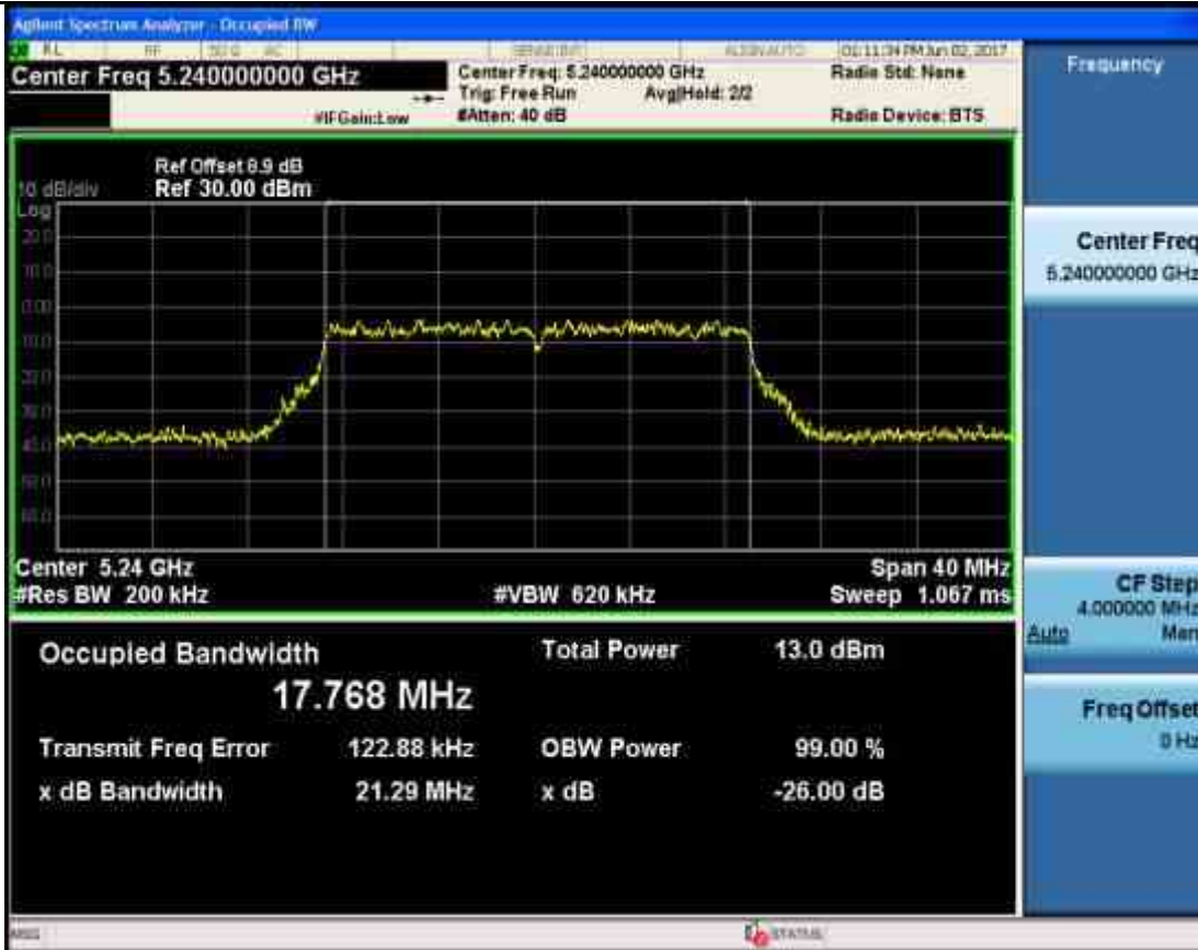
Occupied Bandwidth Measurement_11AC20_5745_Ant1
