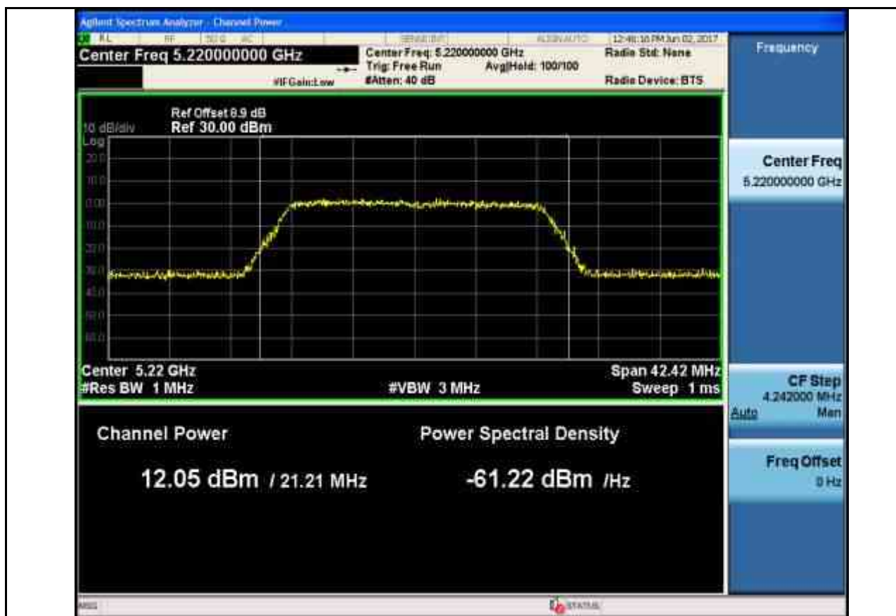
Maximum Conduct Output Power_11N20_5240_Ant1
