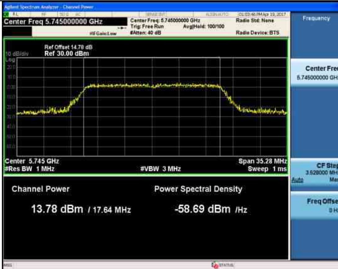
Maximum Conduct Output Power_11N20_5785_Ant2
