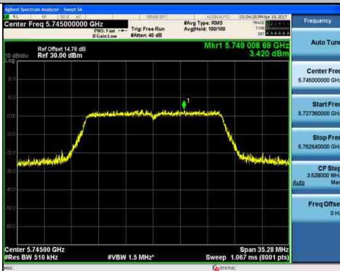
Maximum Conduct Output Power_TNVN_11N20_5785_Ant2
