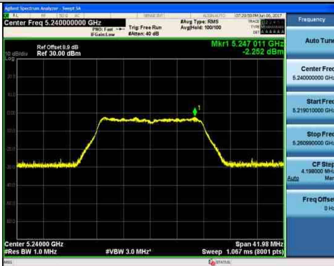
Maximum Conduct Output Power_TNVN_11A_5745_Ant1
