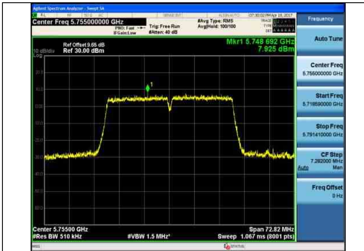
Maximum Conduct Output Power_TNVN_11AC40_5795_Ant1
