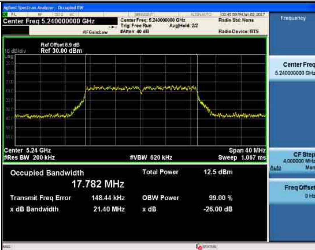
Occupied Bandwidth Measurement_11AC20_5745_Ant2
