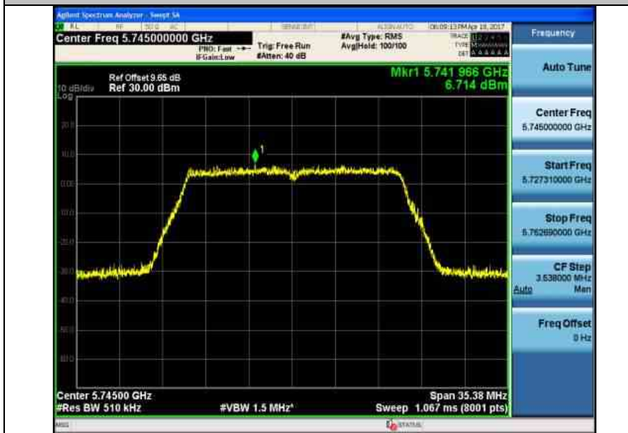
Maximum Conduct Output Power_TNVN_11N20_5785_Ant1
