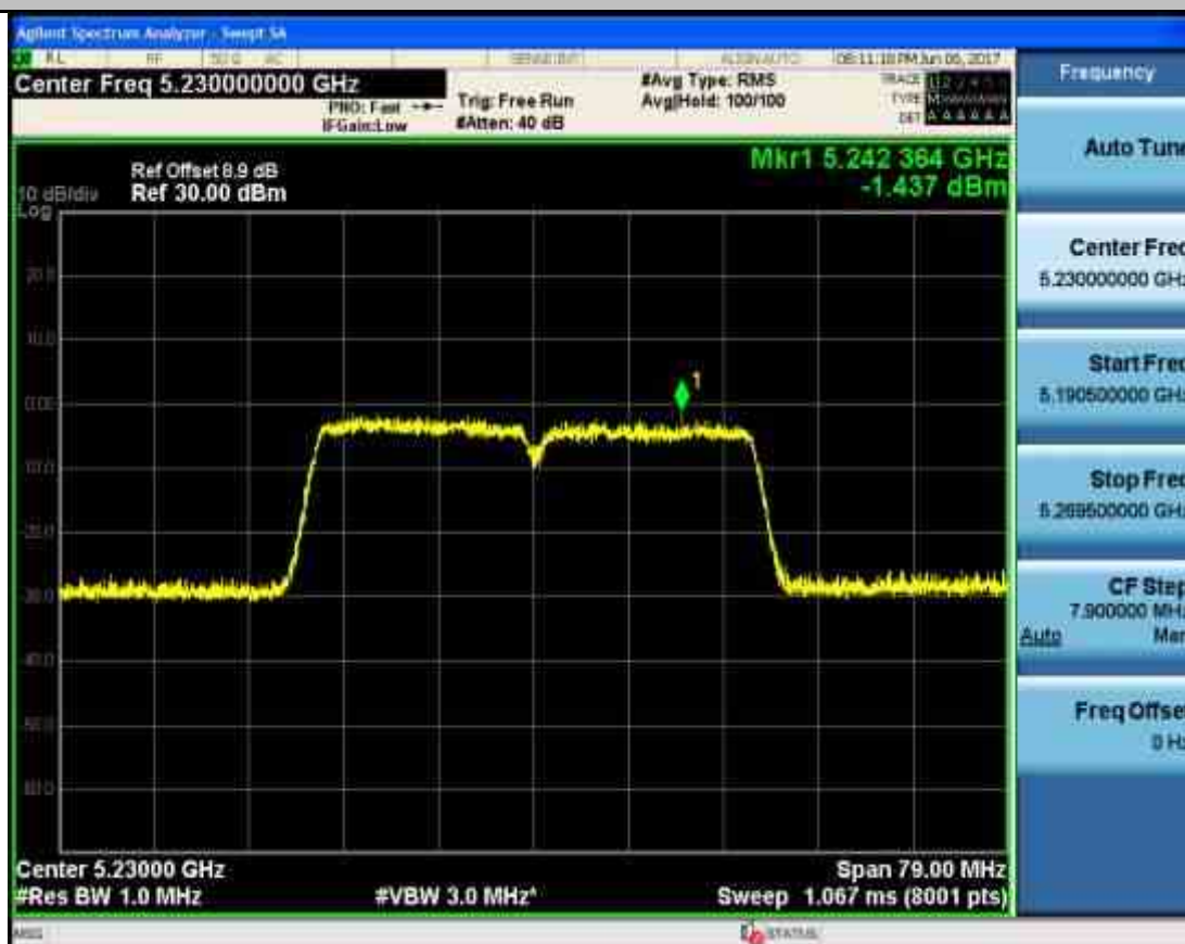
Maximum Conduct Output Power_TNVN_11N40_5755_Ant2
