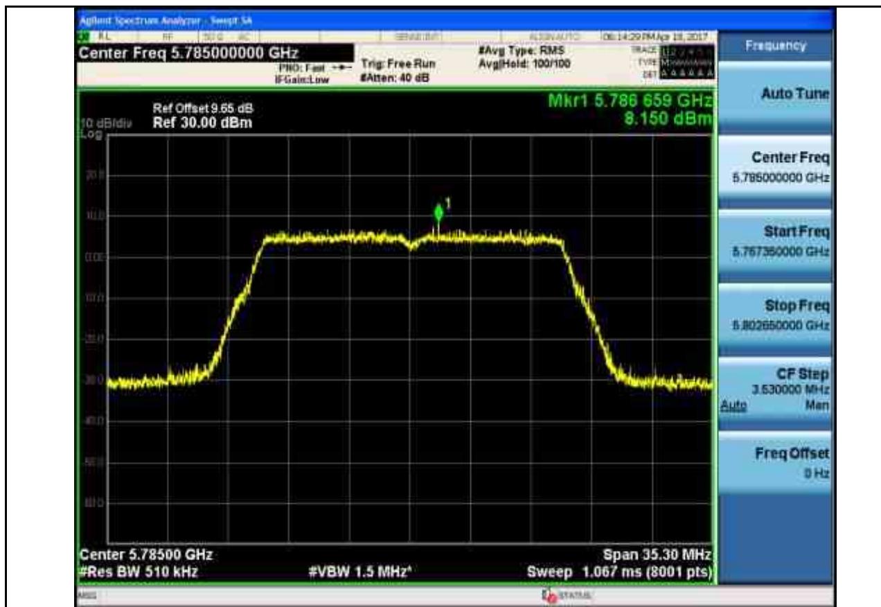
Maximum Conduct Output Power_TNVN_11N20_5825_Ant1
