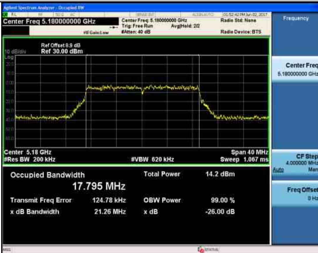
Occupied Bandwidth Measurement_11N20_5220_Ant2
