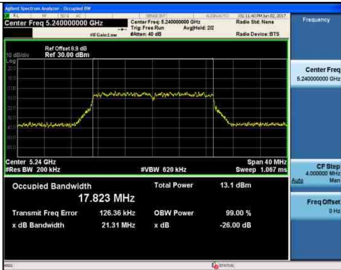
Emission Bandwidth Measurement_11AC20_5745_Ant1
