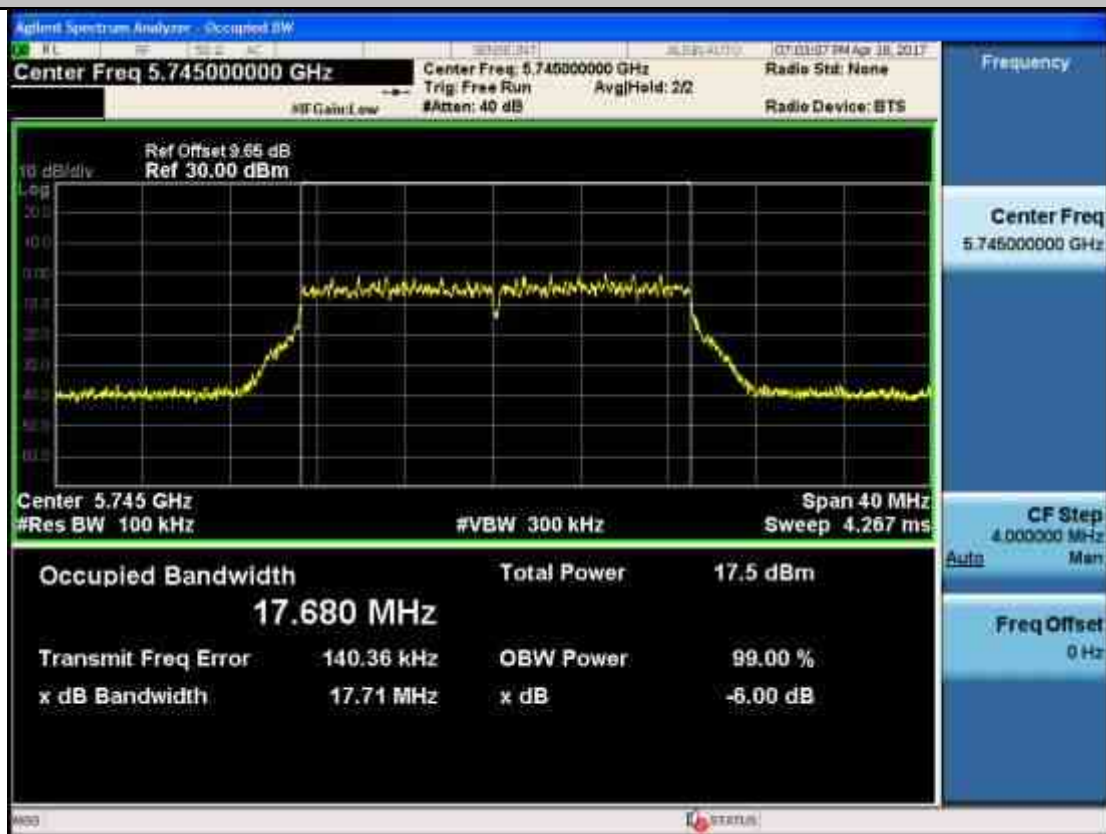
Emission Bandwidth Measurement_11AC20_5745_Ant1
