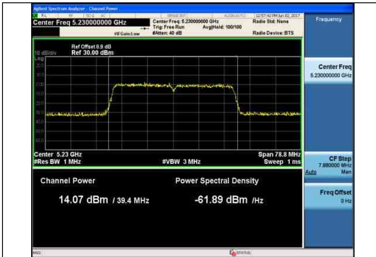
Maximum Conduct Output Power_11N40_5755_Ant1
