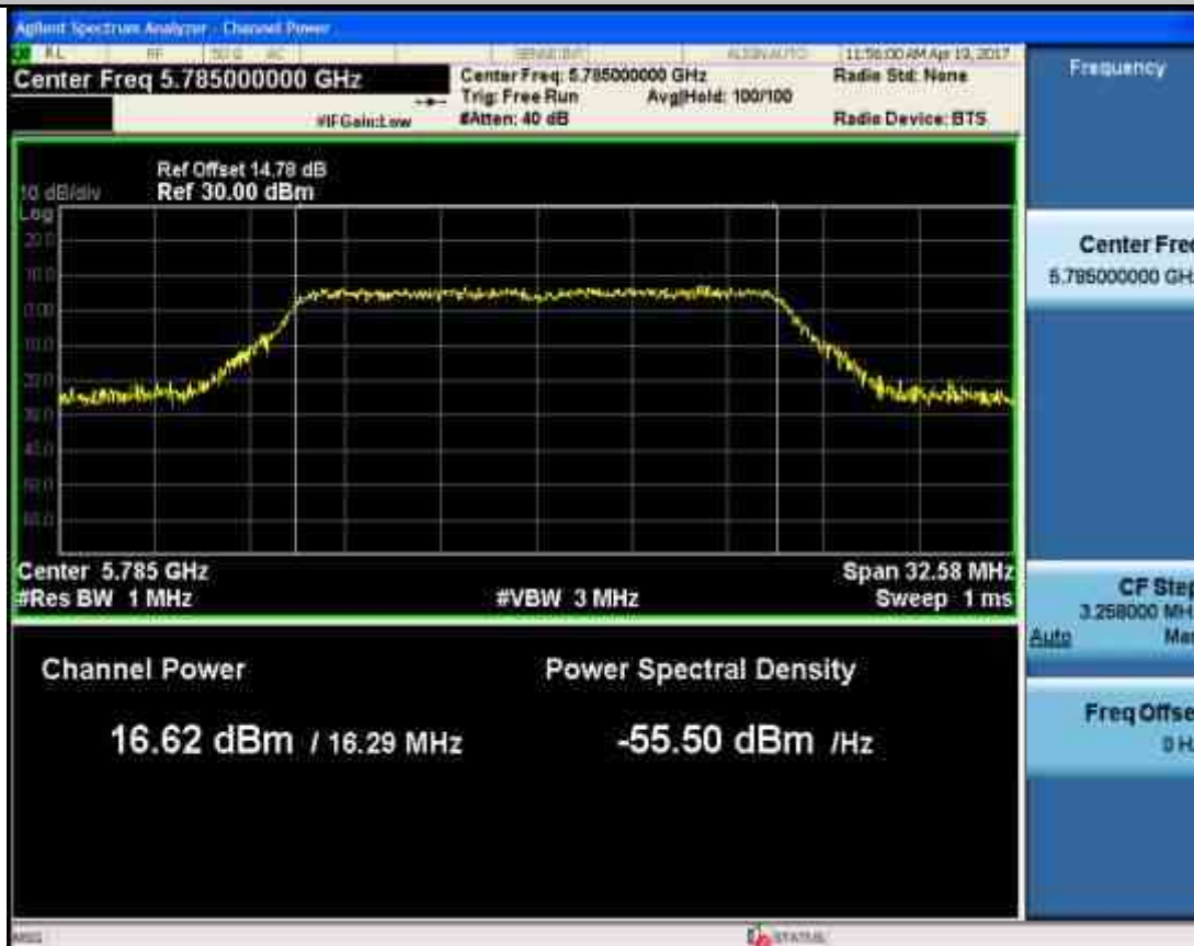
Maximum Conduct Output Power_11A_5825_Ant2
