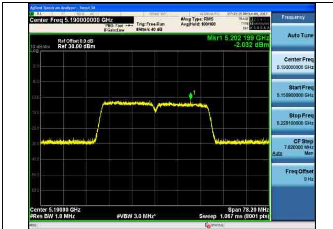
Maximum Conduct Output Power_TNVN_11N40_5230_Ant1
