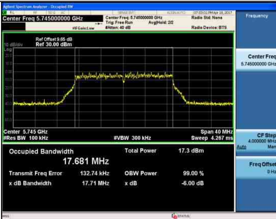
Occupied Bandwidth Measurement_11AC20_5785_Ant1
