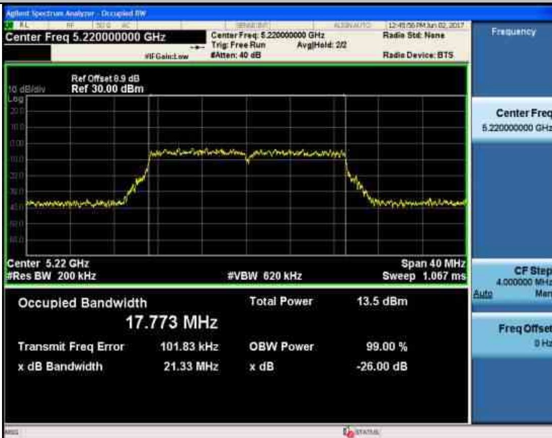
Occupied Bandwidth Measurement_11N20_5240_Ant1
