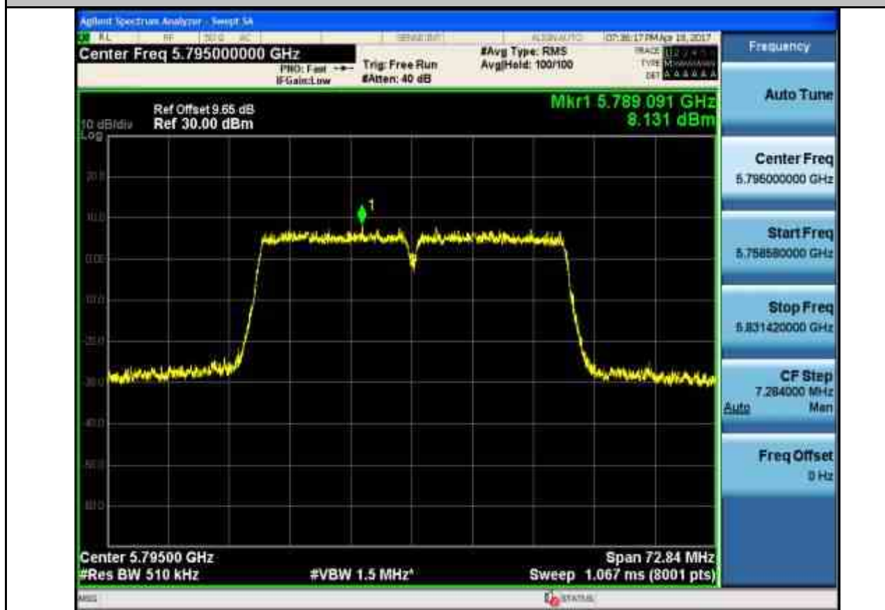
Maximum Conduct Output Power_TNVN_11AC80_5210_Ant1
