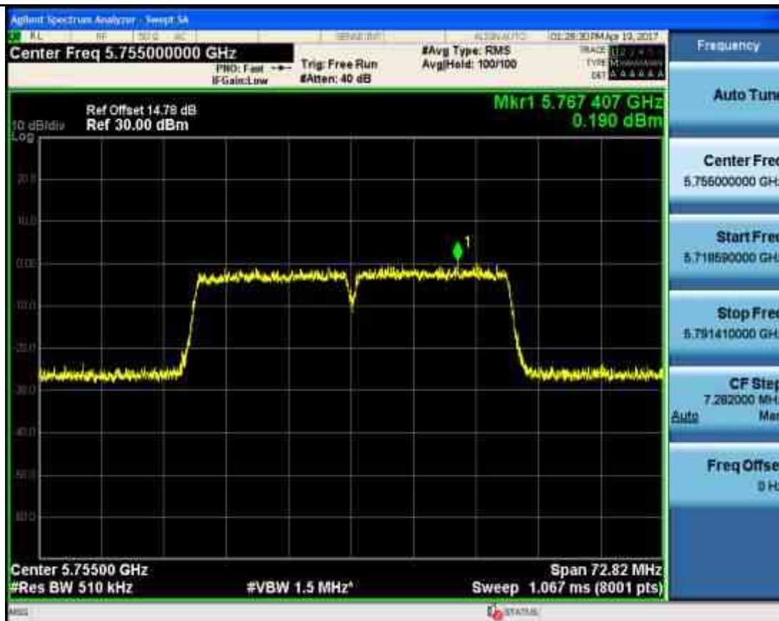
Maximum Conduct Output Power_TNVN_11N40_5795_Ant2
