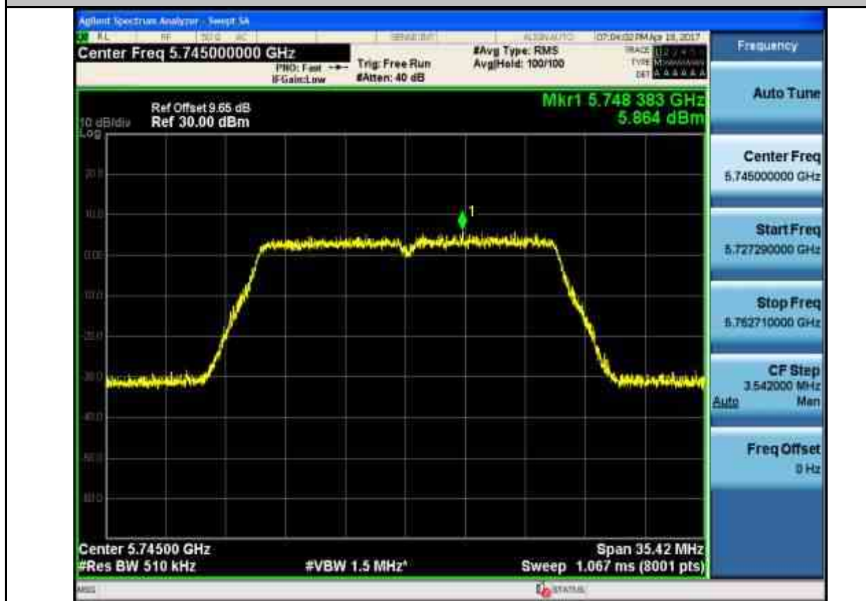
Maximum Conduct Output Power_TNVN_11AC20_5785_Ant1
