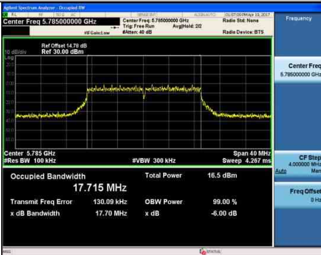
Occupied Bandwidth Measurement_11N20_5825_Ant2
