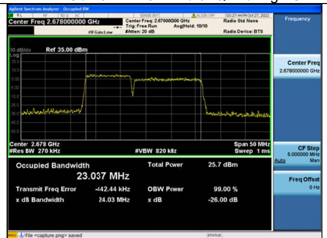
Band41C / 10MHz+15MHz / 16QAM/ High CH
