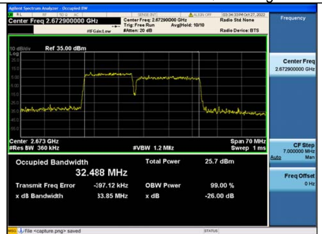
Band41C / 15MHz+20MHz / 64QAM/ High CH
