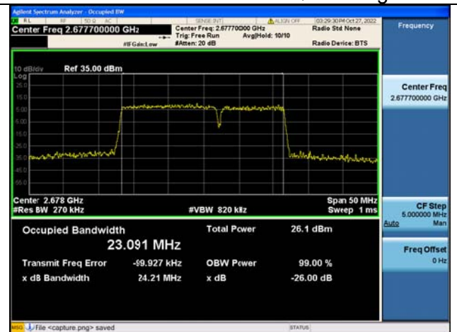
Band41C / 15MHz+10MHz / 64QAM/ High CH
