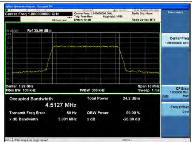
Band2 / 5MHz / 64QAM/ Mid CH
