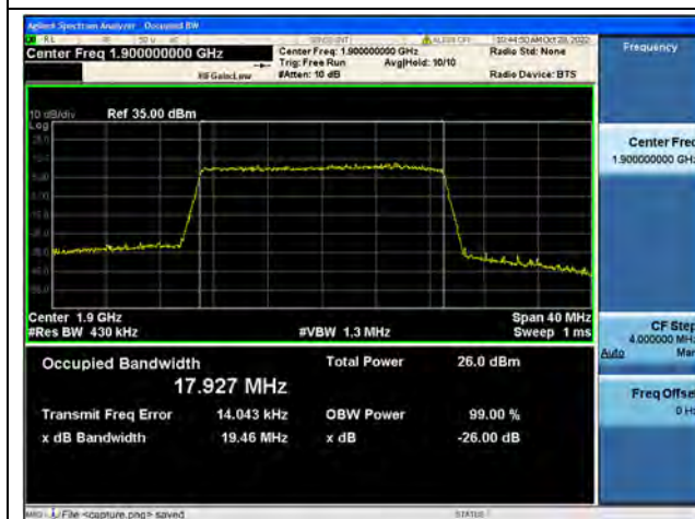
Band2 / 20MHz / 16QAM/ High CH
