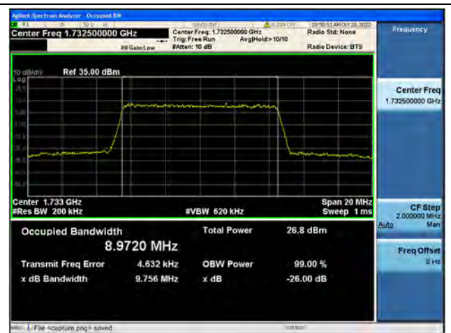
Band4 / 10MHz / 16QAM/ Mid CH
