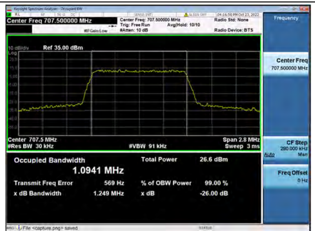
Band12 / 1.4MHz / 64QAM/ Mid CH
