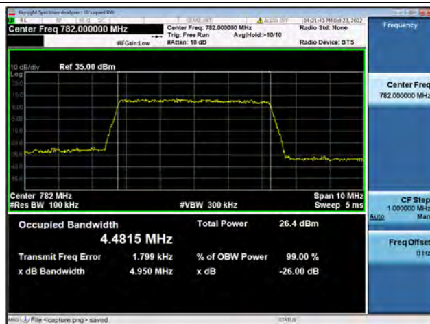
Band13 / 5MHz / 16QAM/ Mid CH
