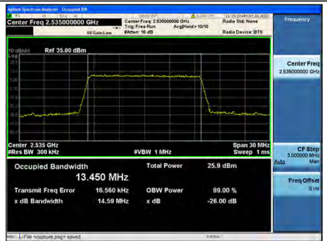
Band7 / 15MHz / QPSK/ Mid CH
