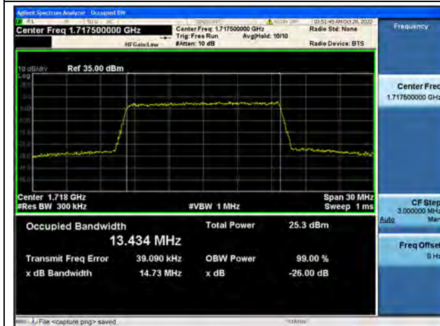
Band4 / 15MHz / 64QAM/ Low CH
