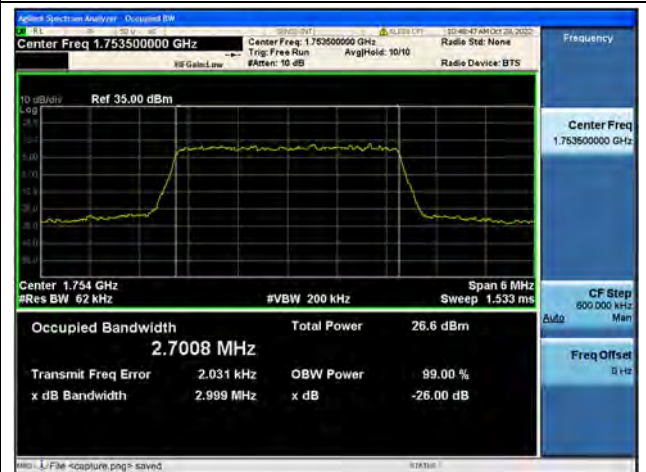
Band4 / 3MHz / QPSK/ High CH
