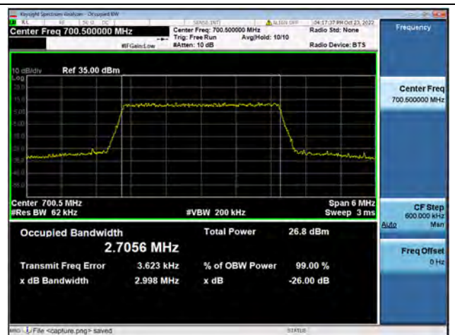
Band12 / 3MHz / 64QAM/ Low CH
