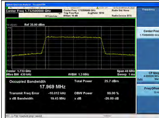
Band4 / 20MHz / 64QAM/ Mid CH
