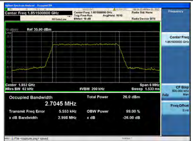
Band25 / 3MHz / QPSK/ Low CH
