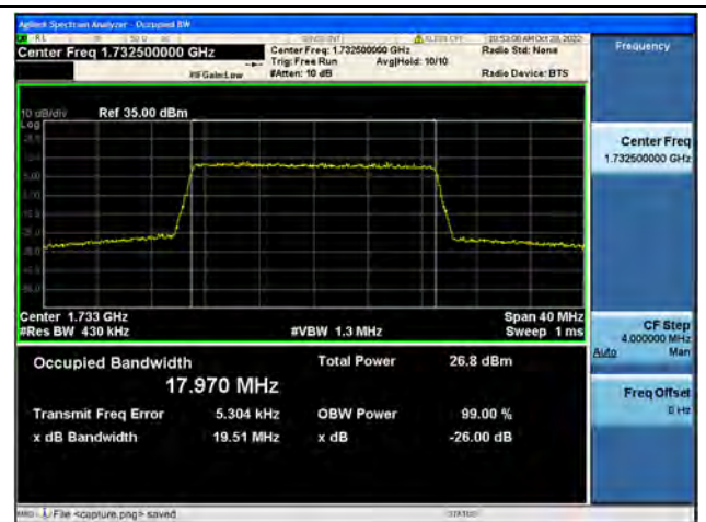
Band4 / 20MHz / 16QAM/ Mid CH
