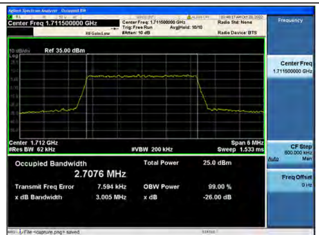
Band4 / 3MHz / 64QAM/ Low CH
