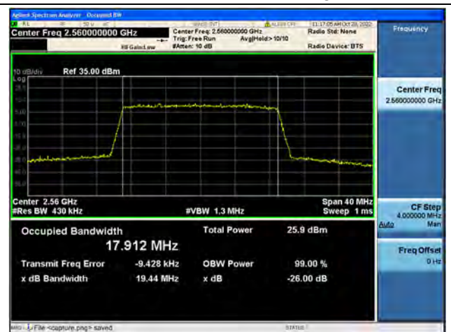
Band7 / 20MHz / 64QAM/ High CH
