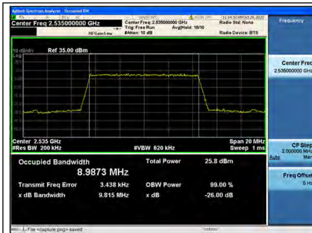
Band7 / 10MHz / QPSK/ Mid CH
