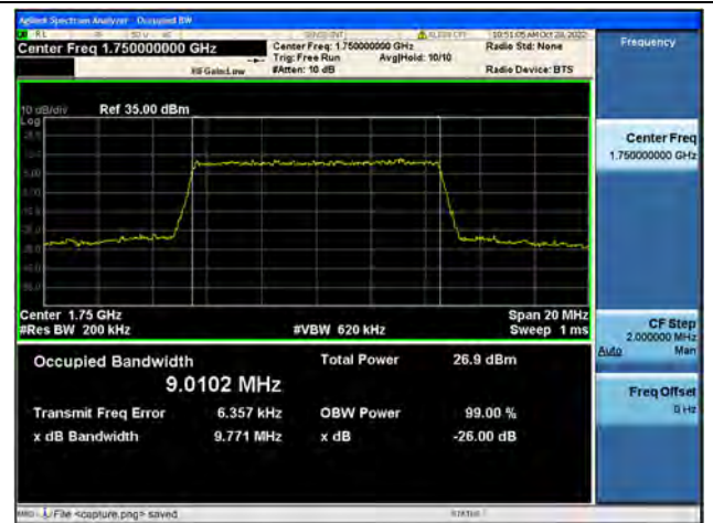
Band4 / 10MHz / QPSK/ High CH
