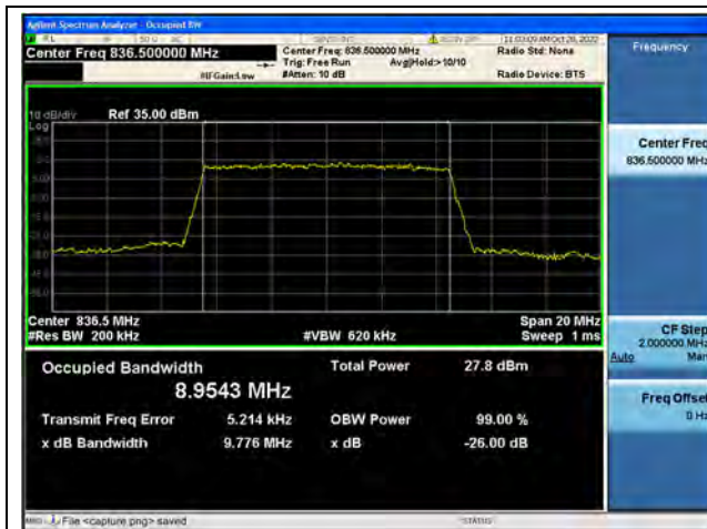
Band5 / 10MHz / QPSK/ Mid CH
