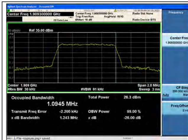
Band2 / 1.4MHz / QPSK/ High CH
