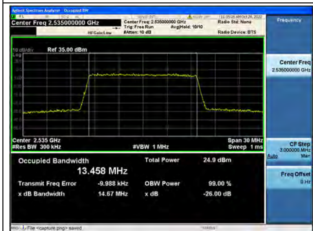
Band7 / 15MHz / 16QAM/ Mid CH
