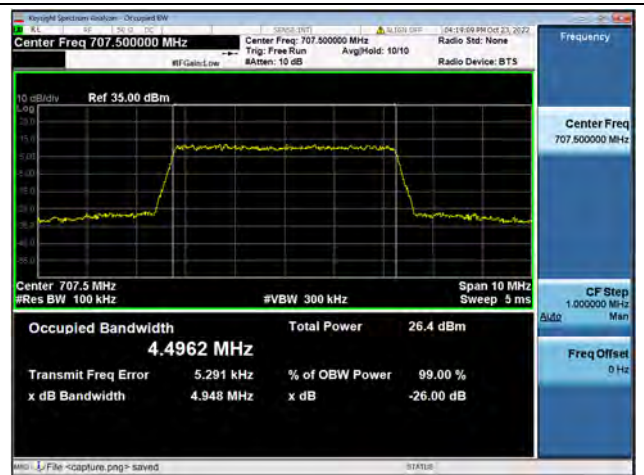
Band12 / 5MHz / 64QAM/ Mid CH
