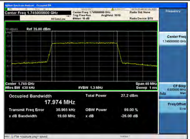
Band4 / 20MHz / QPSK/ High CH
