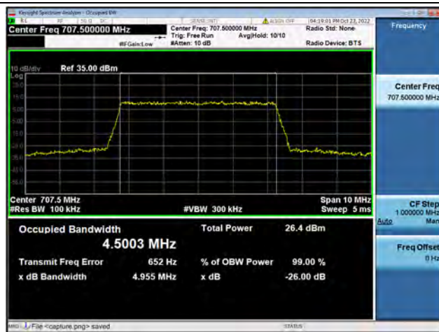
Band12 / 5MHz / 16QAM/ Mid CH
