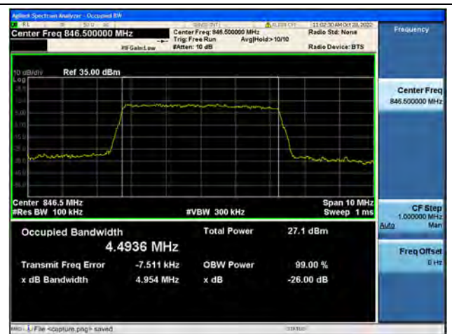
Band5 / 5MHz / 16QAM/ High CH
