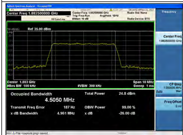
Band25 / 5MHz / 16QAM/ Mid CH
