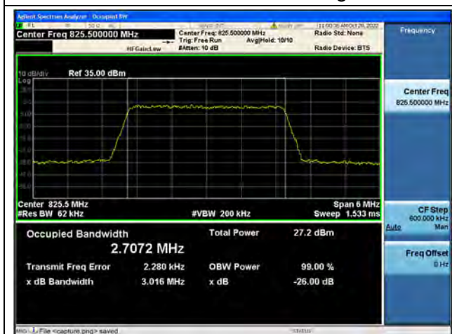
Band5 / 3MHz / 16QAM/ Low CH
