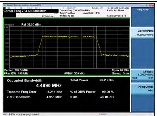
Band13 / 5MHz / 16QAM/ High CH
