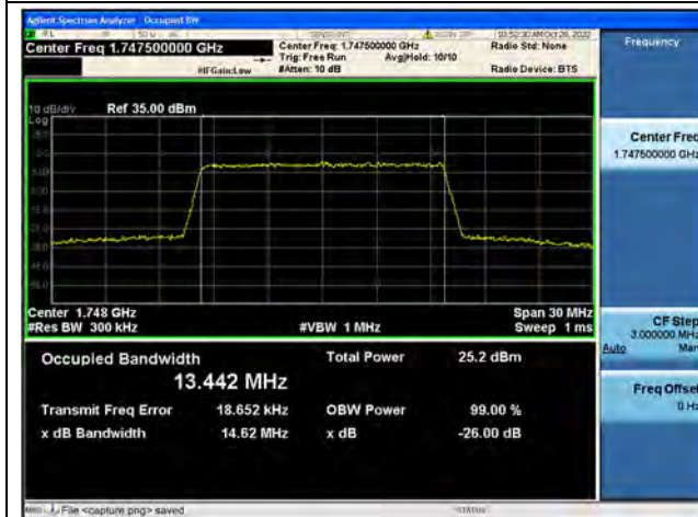
Band4 / 15MHz / 64QAM/ High CH
