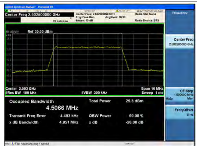
Band7 / 5MHz / 16QAM/ Low CH
