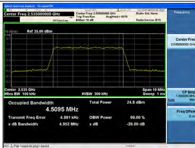
Band7 / 5MHz / 16QAM/ Mid CH
