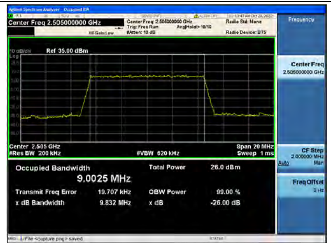
Band7 / 10MHz / QPSK/ Low CH
