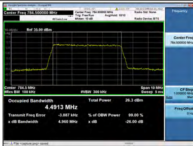
Band13 / 5MHz / 64QAM/ High CH
