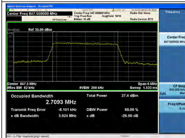
Band5 / 3MHz / 16QAM/ High CH
