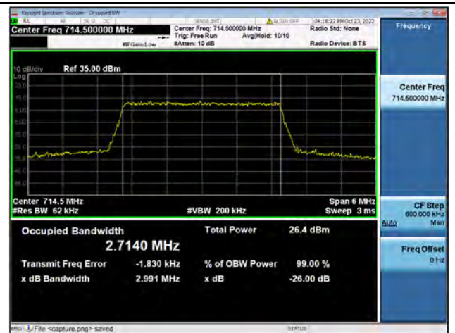
Band12 / 3MHz / 64QAM/ High CH
