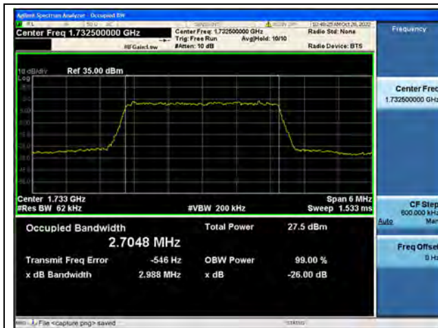
Band4 / 3MHz / QPSK/ Mid CH
