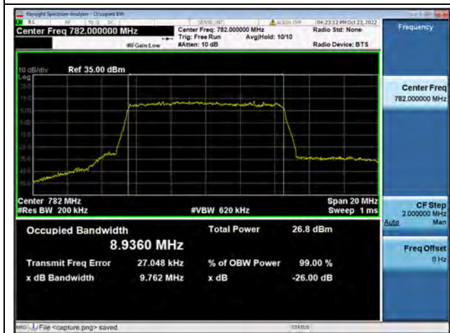
Band13 / 10MHz / 16QAM/ High CH
