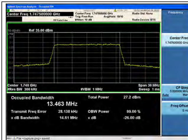
Band4 / 15MHz / QPSK/ High CH
