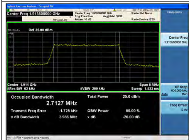
Band25 / 3MHz / 16QAM/ High CH
