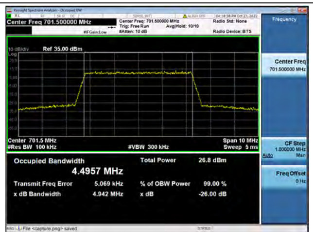
Band12 / 5MHz / 16QAM/ Low CH
