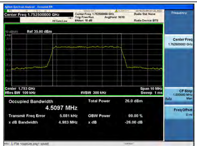
Band4 / 5MHz / 16QAM/ High CH
