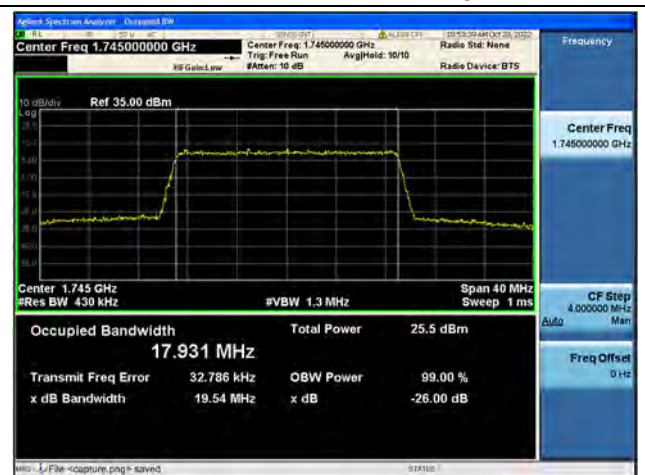
Band4 / 20MHz / 64QAM/ High CH
