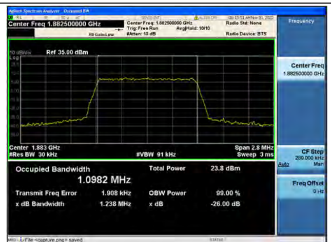
Band25 / 1.4MHz / 64QAM/ Mid CH
