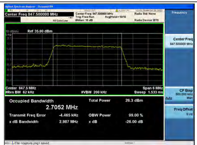
Band5 / 3MHz / 64QAM/ High CH
