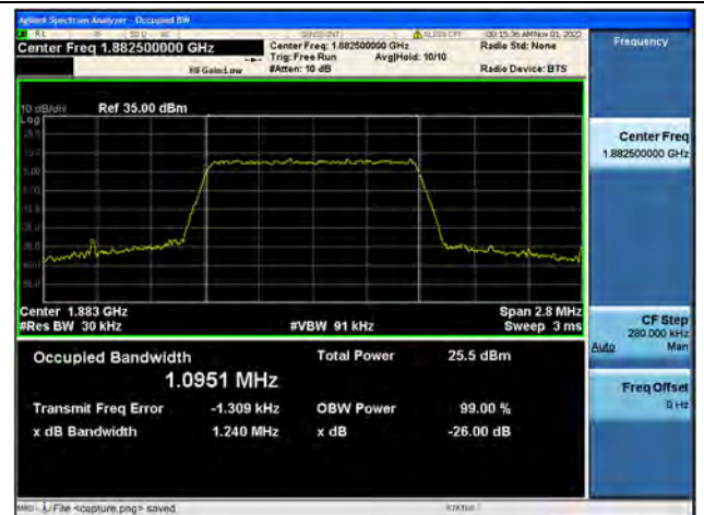
Band25 / 1.4MHz / QPSK/ Mid CH
