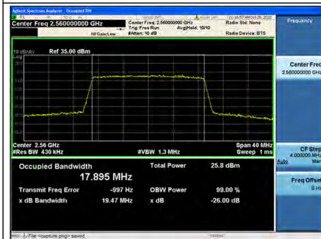
Band7 / 20MHz / 16QAM/ High CH
