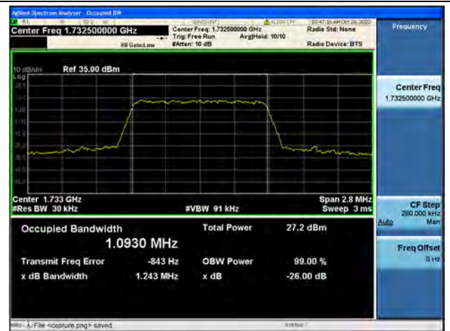
Band4 / 1.4MHz / QPSK/ Mid CH
