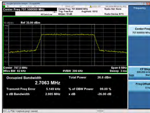
Band12 / 3MHz / 64QAM/ Mid CH
