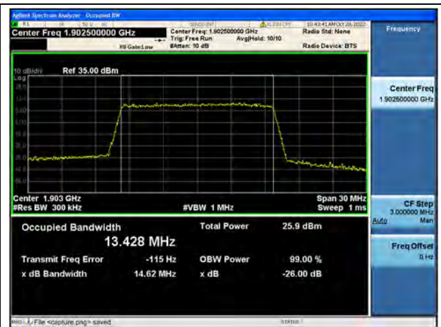
Band2 / 15MHz / 16QAM/ High CH
