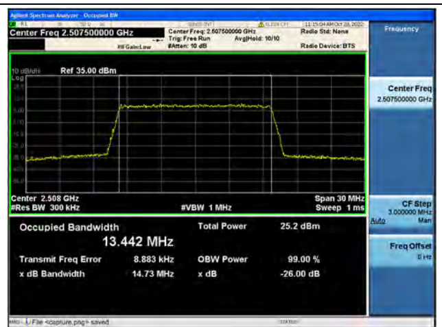
Band7 / 15MHz / 16QAM/ Low CH
