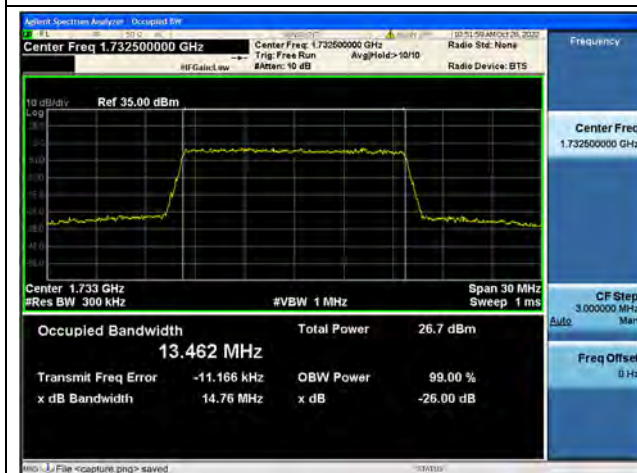
Band4 / 15MHz / 16QAM/ Mid CH
