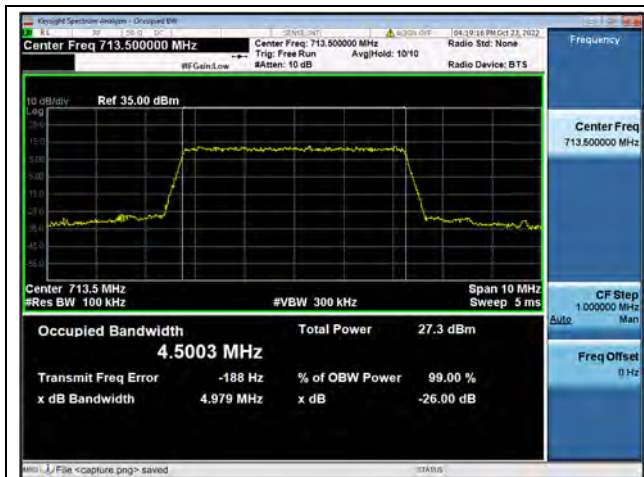
Band12 / 5MHz / QPSK/ High CH
