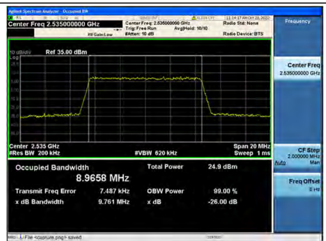
Band7 / 10MHz / 16QAM/ Mid CH
