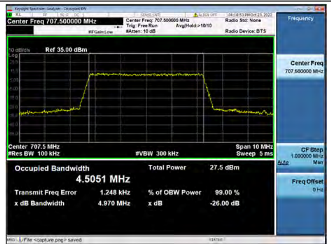
Band12 / 5MHz / QPSK/ Mid CH
