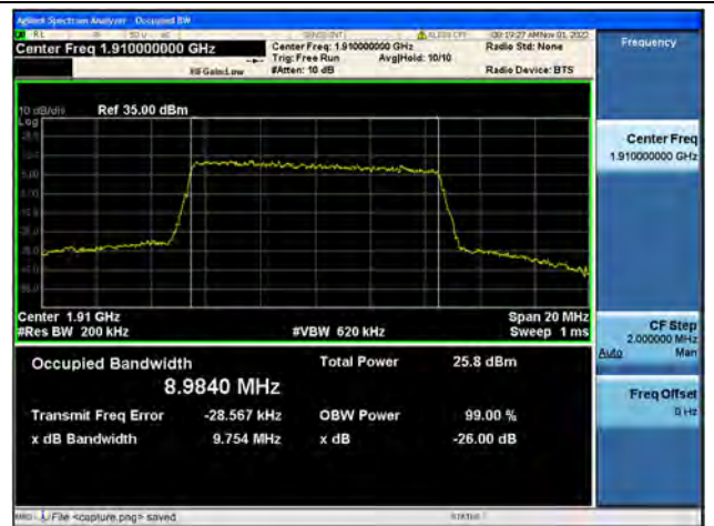
Band25 / 10MHz / QPSK/ High CH
