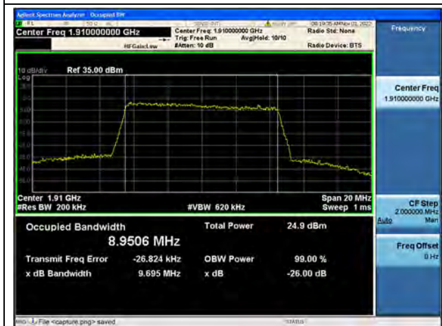
Band25 / 10MHz / 16QAM/ High CH
