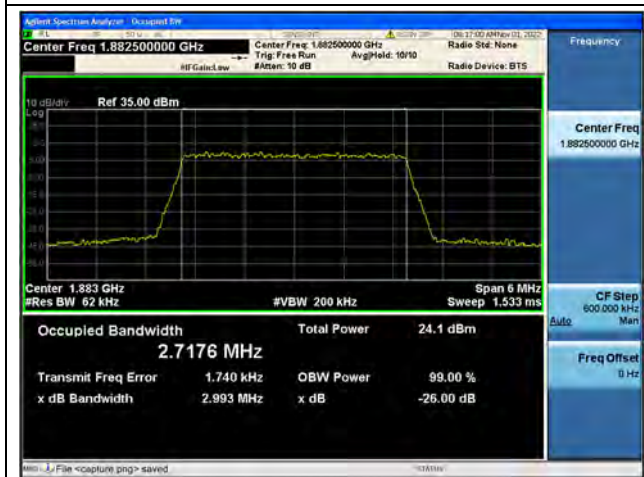
Band25 / 3MHz / 64QAM/ Mid CH
