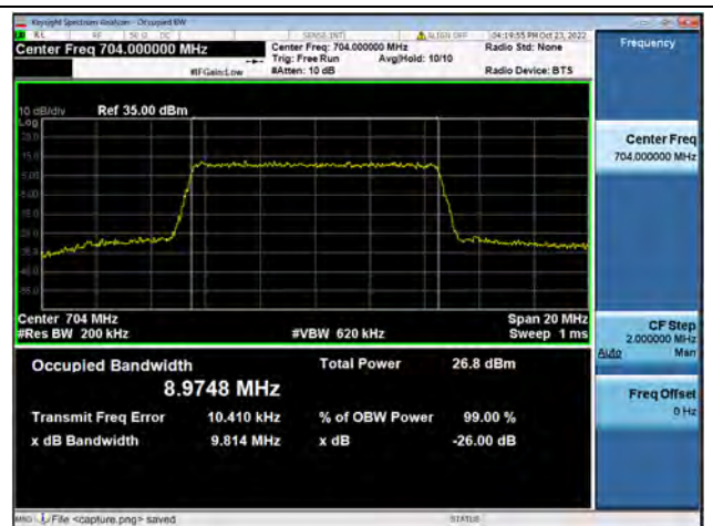
Band12 / 10MHz / 64QAM/ Low CH
