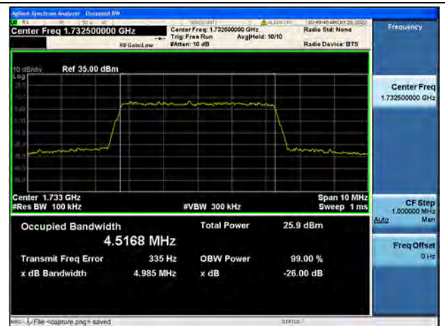
Band4 / 5MHz / 64QAM/ Mid CH
