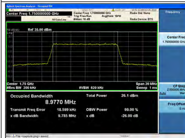
Band4 / 10MHz / 16QAM/ High CH
