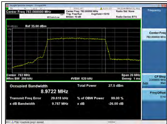
Band13 / 10MHz / QPSK/ Mid CH
