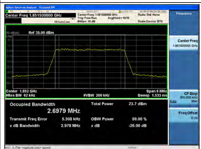
Band2 / 3MHz / 64QAM/ Low CH
