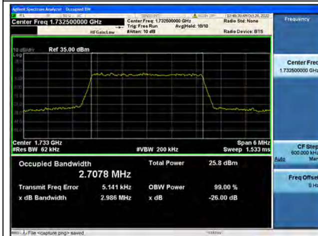
Band4 / 3MHz / 64QAM/ Mid CH
