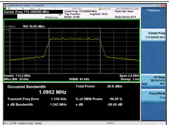
Band12 / 1.4MHz / 16QAM/ High CH
