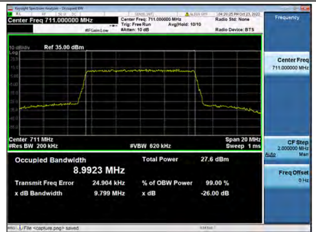
Band12 / 10MHz / QPSK/ High CH
