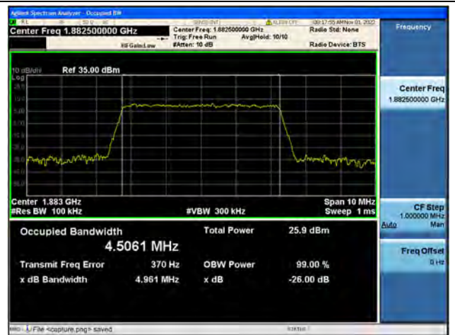
Band25 / 5MHz / QPSK/ Mid CH
