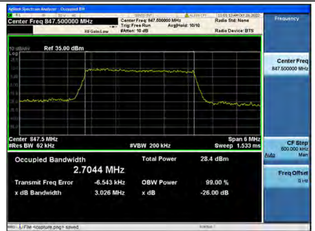
Band5 / 3MHz / QPSK/ High CH
