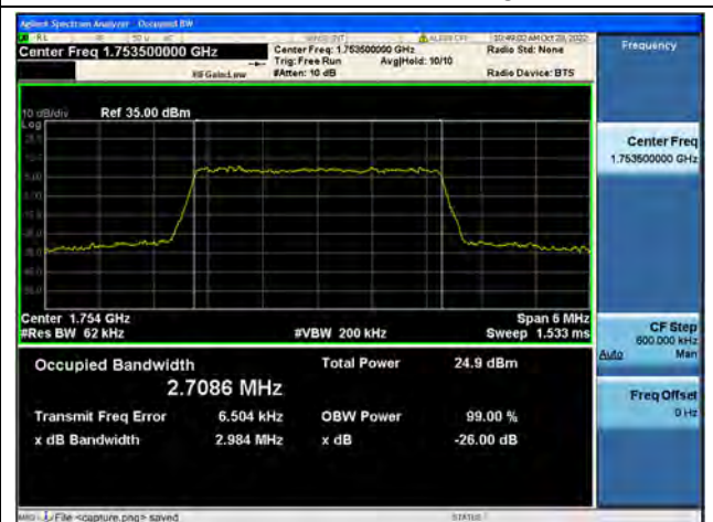
Band4 / 3MHz / 64QAM/ High CH
