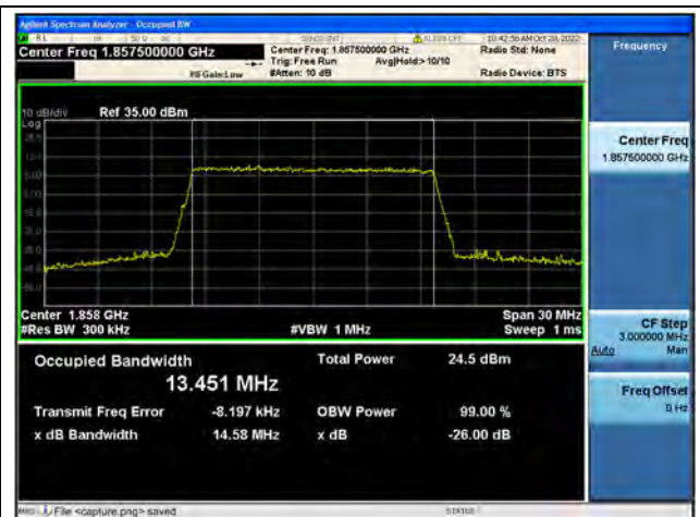
Band2 / 15MHz / 16QAM/ Low CH
