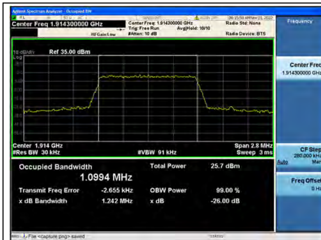
Band25 / 1.4MHz / QPSK/ High CH
