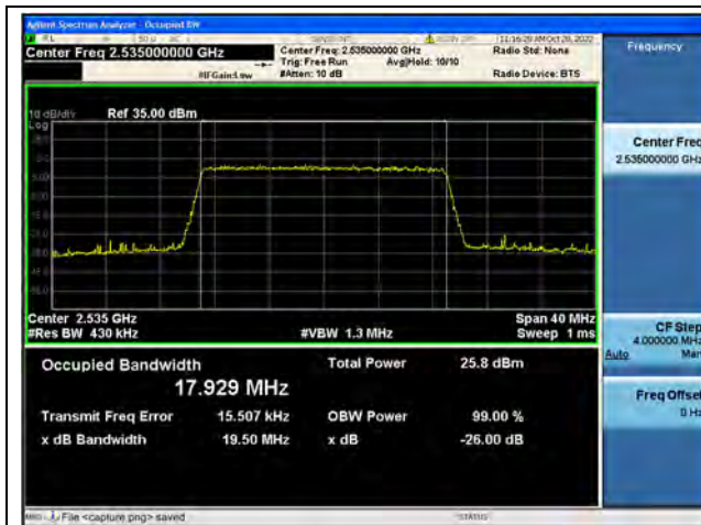
Band7 / 20MHz / QPSK/ Mid CH
