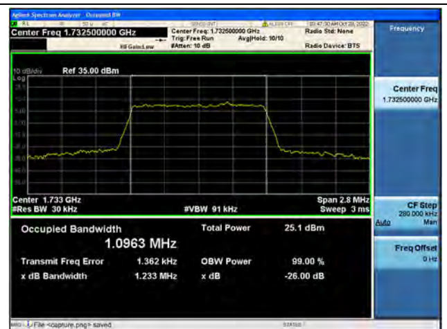
Band4 / 1.4MHz / 64QAM/ Mid CH
