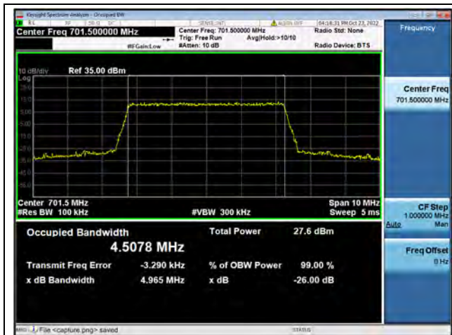
Band12 / 5MHz / QPSK/ Low CH
