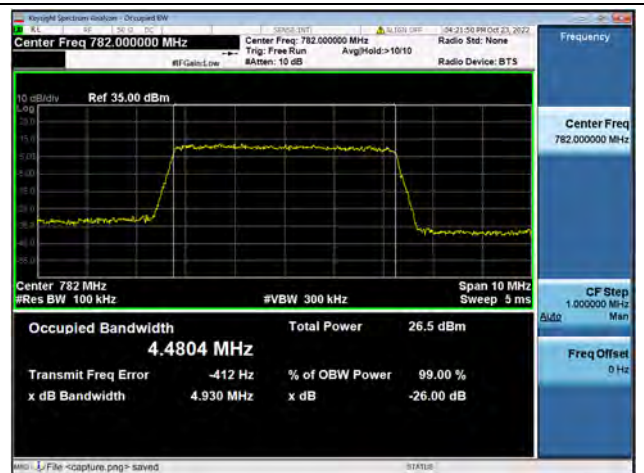
Band13 / 5MHz / 64QAM/ Mid CH
