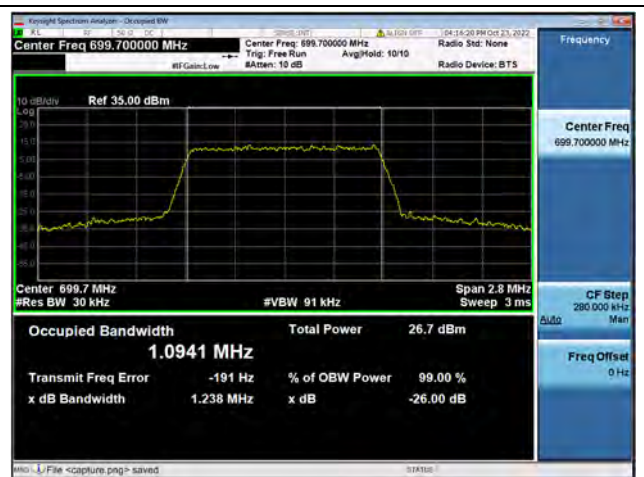
Band12 / 1.4MHz / 16QAM/ Low CH
