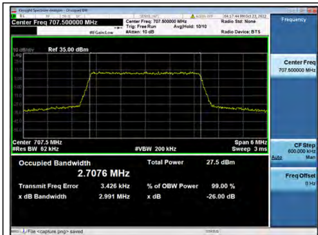
Band12 / 3MHz / QPSK/ Mid CH
