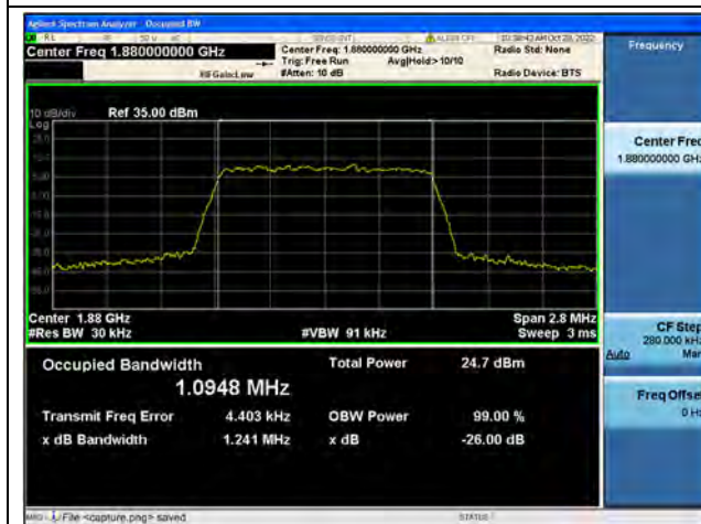
Band2 / 1.4MHz / 16QAM/ Mid CH
