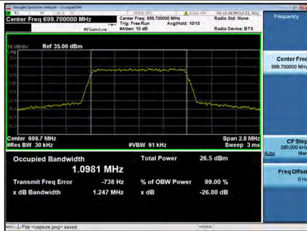
Band12 / 1.4MHz / 64QAM/ Low CH
