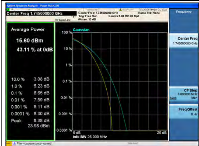
Band66 / 20MHz / Mid CH / 64QAM
