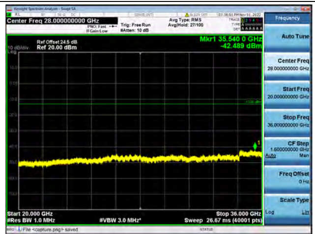
Band42-20G-36G / 15MHz / Low CH / QPSK
