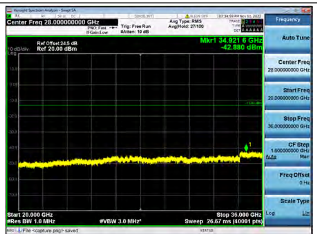
Band42-20G-36G / 10MHz / Low CH / QPSK
