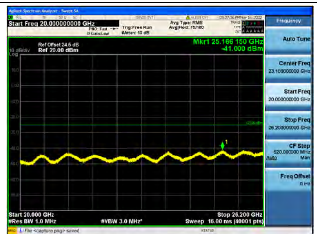
Band38-20G-26G / 15MHz / Low CH / QPSK
