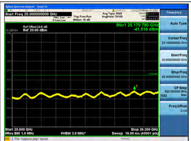
Band38-20G-26G / 20MHz / Low CH / QPSK
