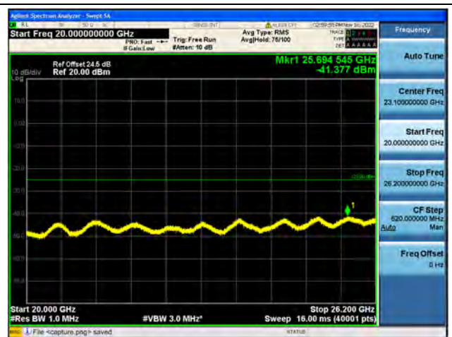
Band38-20G-26G / 5MHz / Low CH / QPSK
