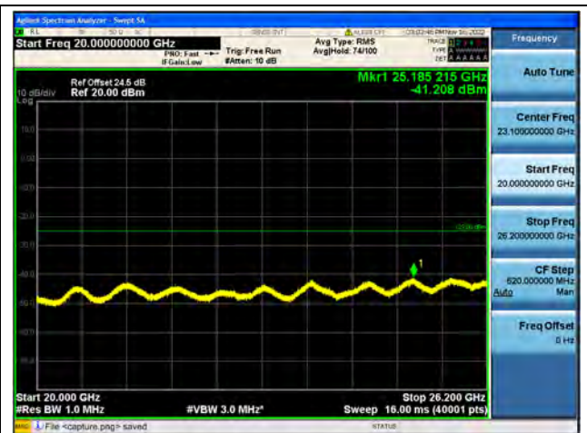
Band38-20G-26G / 10MHz / Low CH / QPSK
