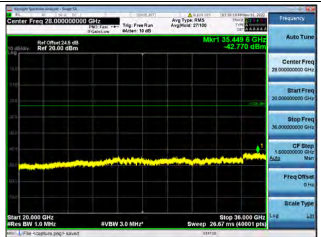
Band42-20G-36G / 5MHz / Low CH / QPSK
