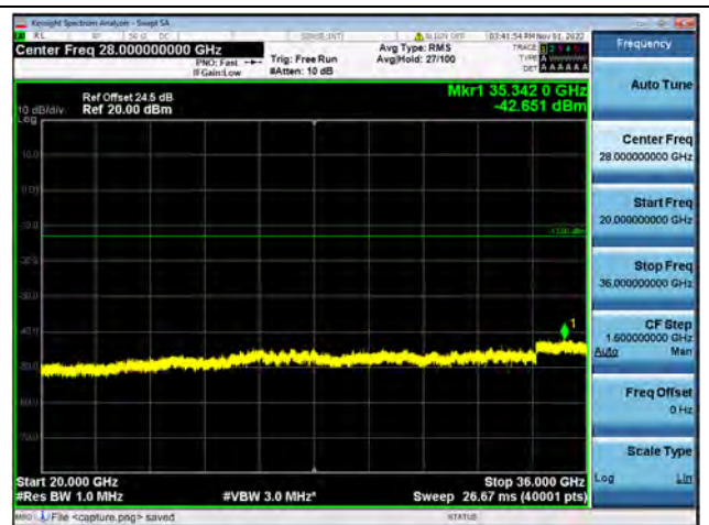
Band42-20G-36G / 20MHz / Low CH / QPSK
