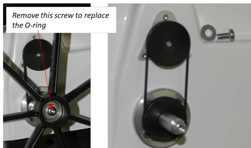
Figure 5, Removing the wheel and replacing the O-ring
