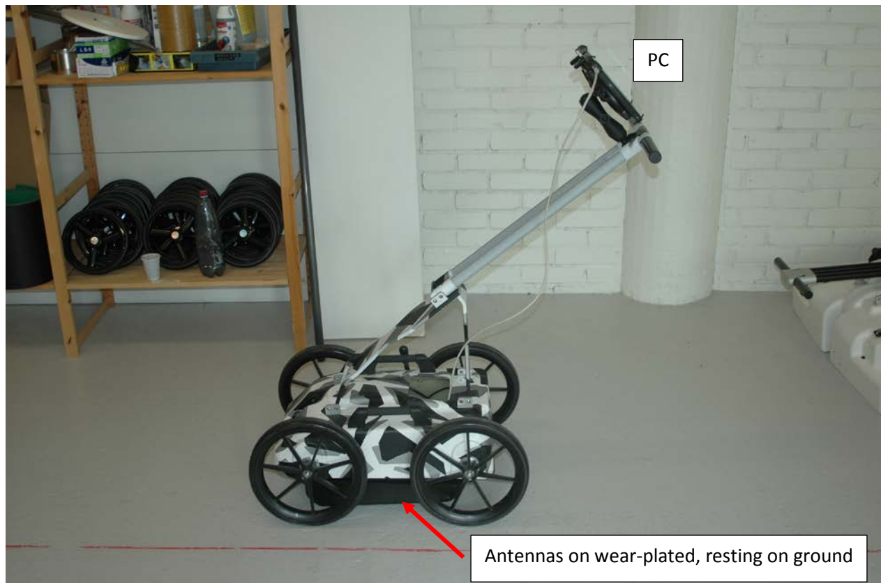
Example configuration, ready for operation. Antennas placed on wear-plate directed towards ground, and wear plate hooked up to trolley.
