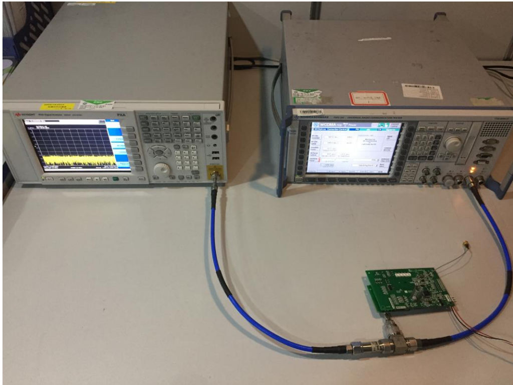
Photograph 2: Set-up for Conducted testing
