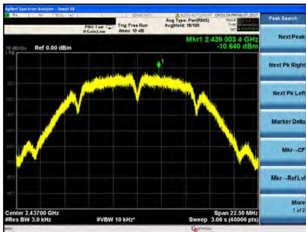
(802.11b) PSD plot on channel 6
