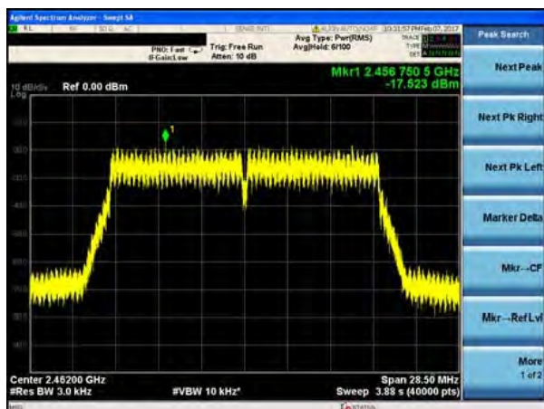
(802.11n20) PSD plot on channel 11
