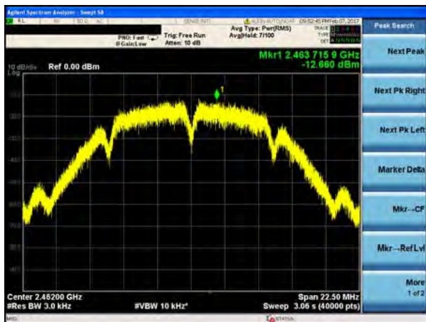
(802.11b) PSD plot on channel 11
