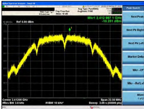
(802.11b) PSD plot on channel 6
