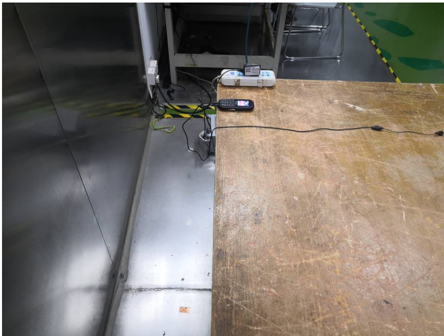
Conducted Emissions - Side View
