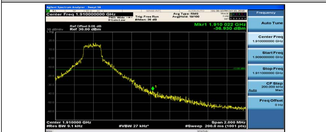
(Channel Bandwidth: 1.4 MHz)_HCH_QPSK_1RB#5
