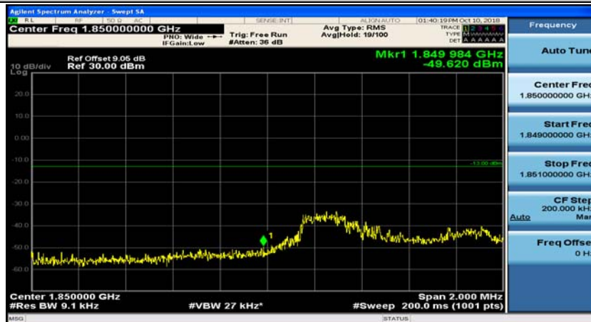
(Channel Bandwidth: 3 MHz)_LCH_16QAM_8RB#0
