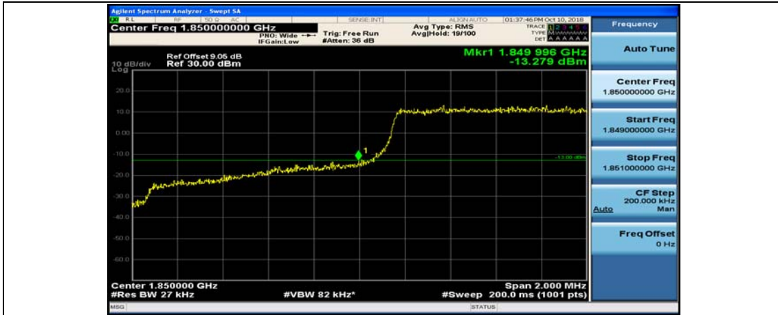
(Channel Bandwidth: 1.4 MHz)_HCH_QPSK_1RB#0
