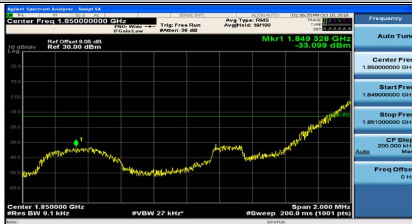
(Channel Bandwidth: 1.4 MHz)_LCH_QPSK_1RB#5
