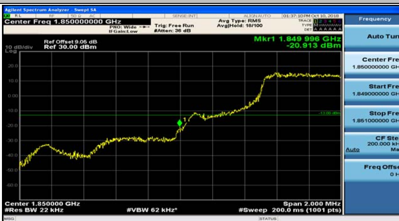
(Channel Bandwidth: 1.4 MHz)_LCH_QPSK_3RB#3
