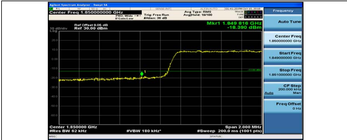
(Channel Bandwidth: 3 MHz)_HCH_16QAM_1RB#0
