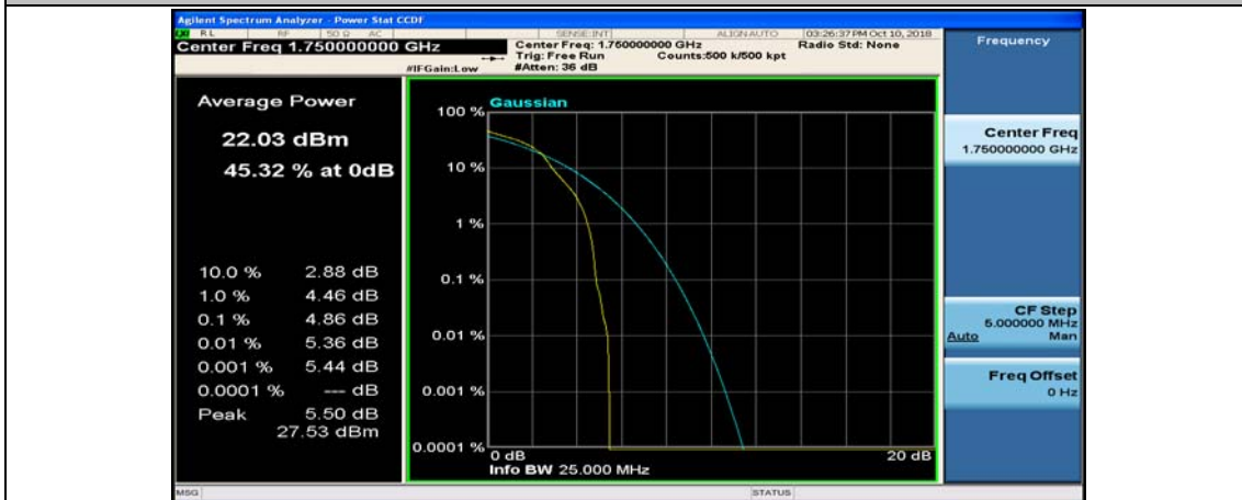
Channel Bandwidth: 10 MHz_HCH_16QAM_1RB#24
