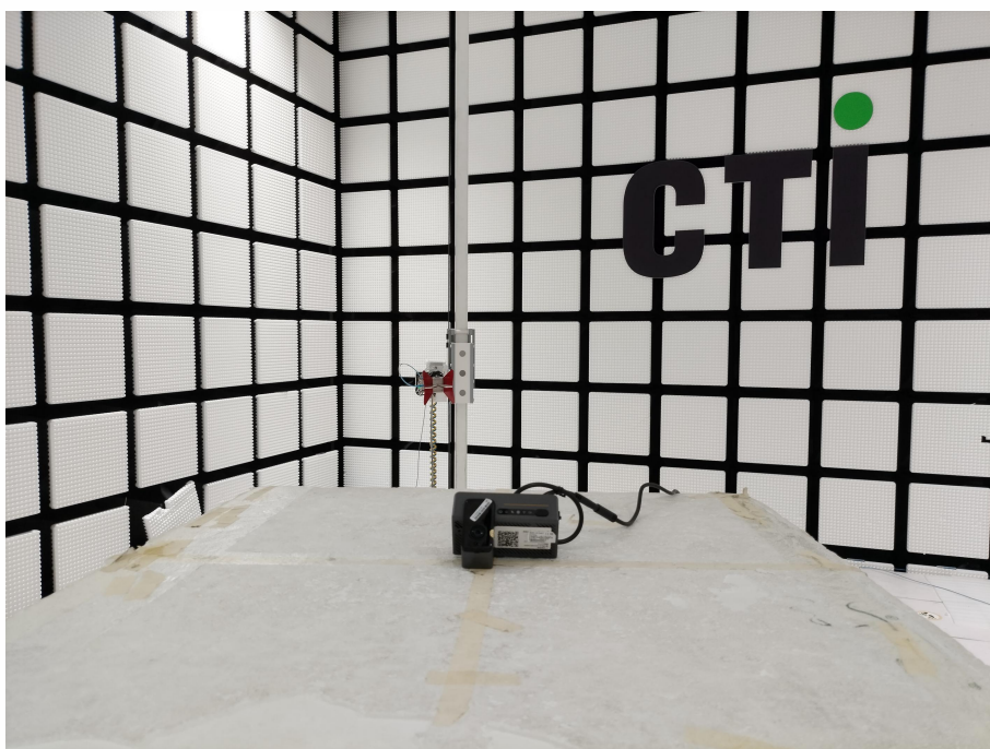
Radiated spurious emission Test Setup-2(Above 1GHz)
