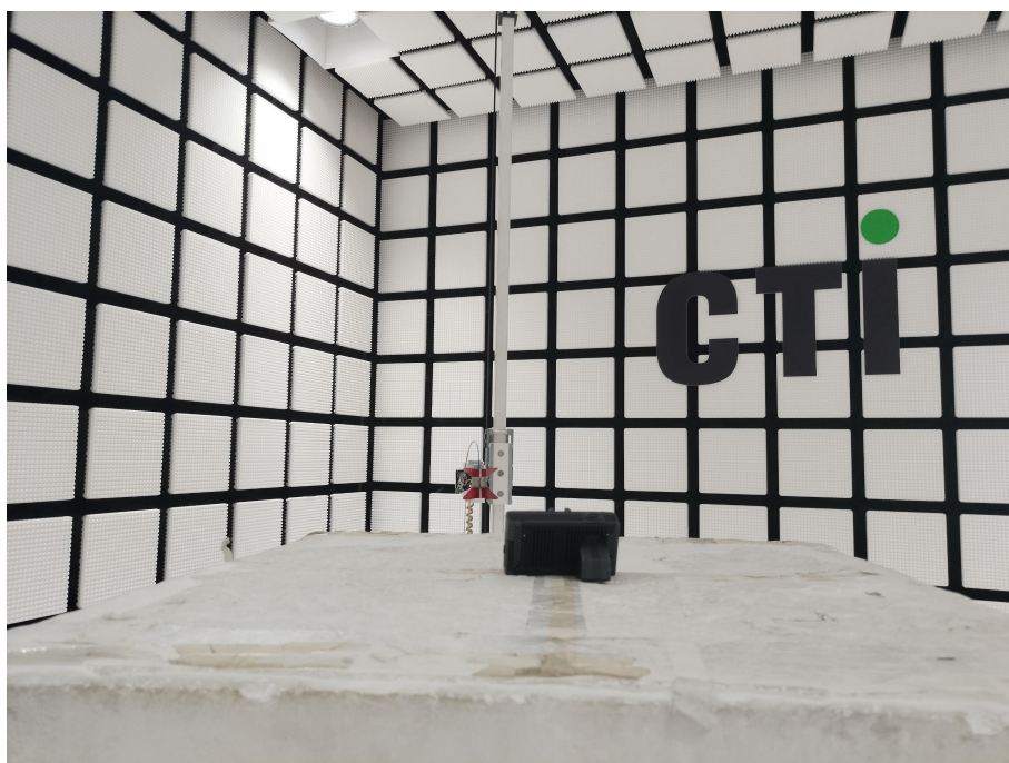
Radiated spurious emission Test Setup-2(Above 1GHz)
