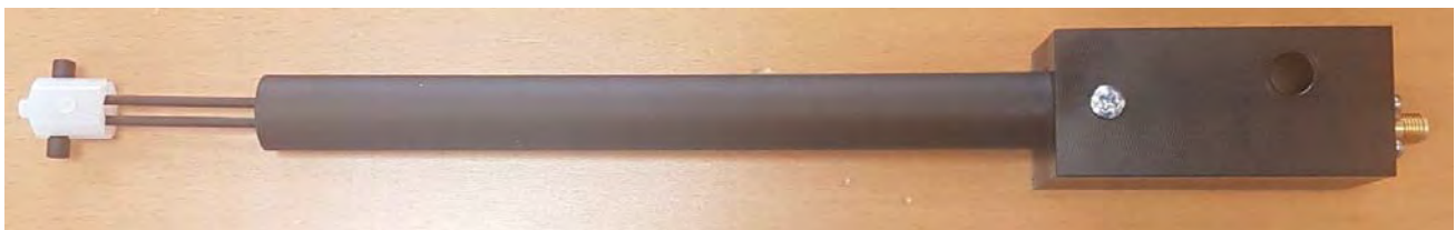
Figure 1 – MVG COMOSAR Validation Dipole
