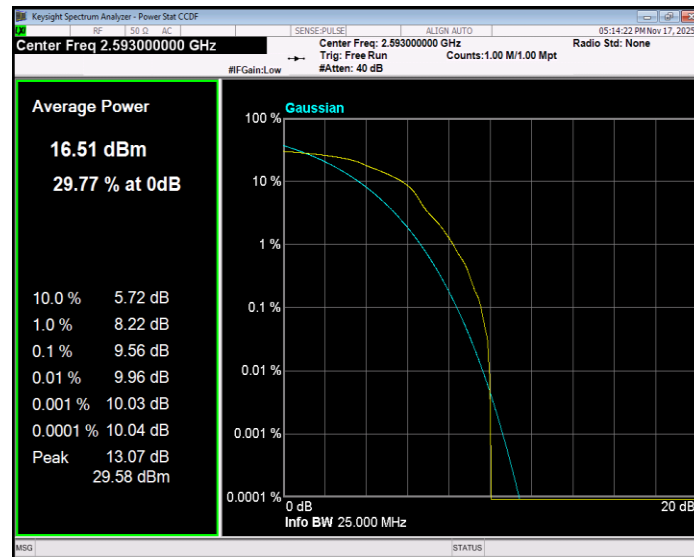
Band41 16QAM BW=5MHz Channel=41565 RB Size=1 Position=#0
