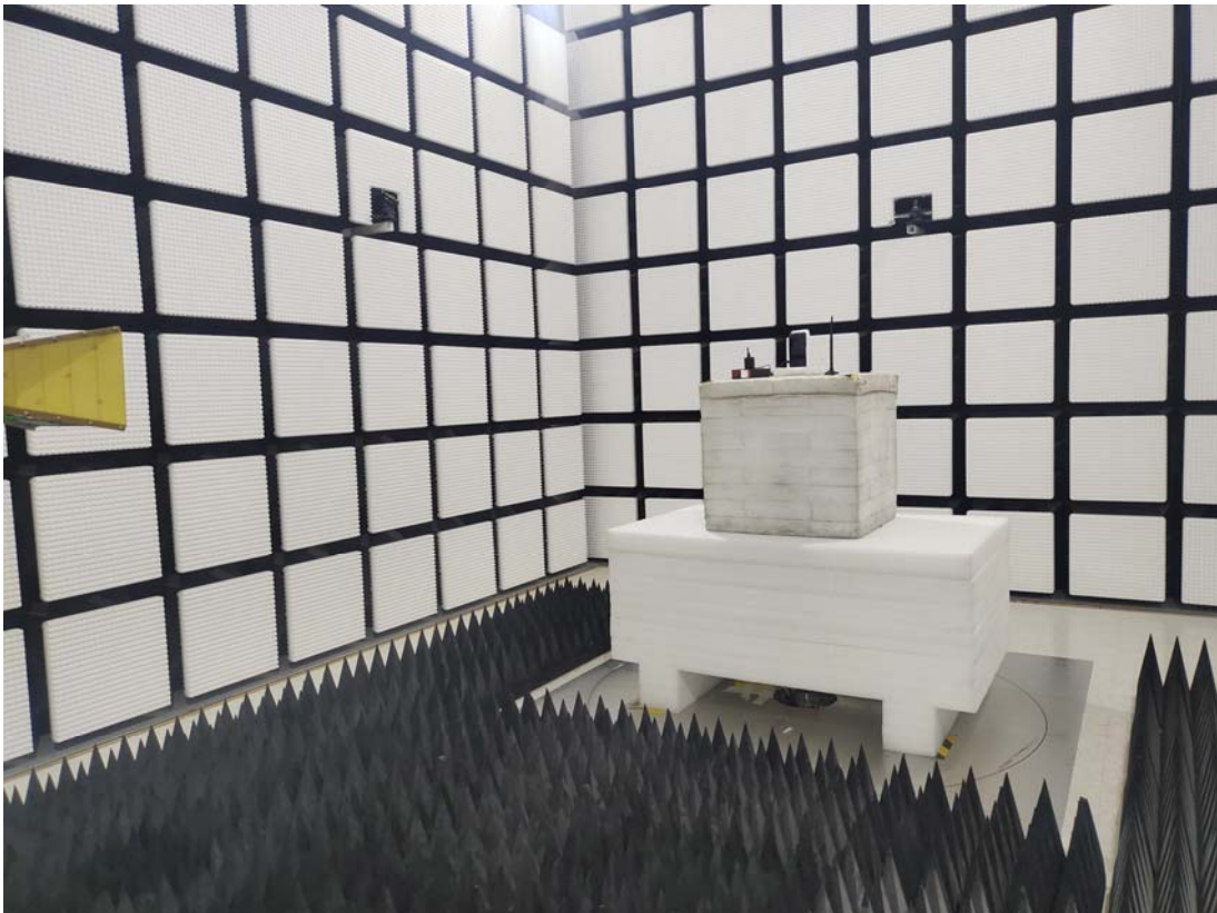
Radiated Emission Above 1GHz View
