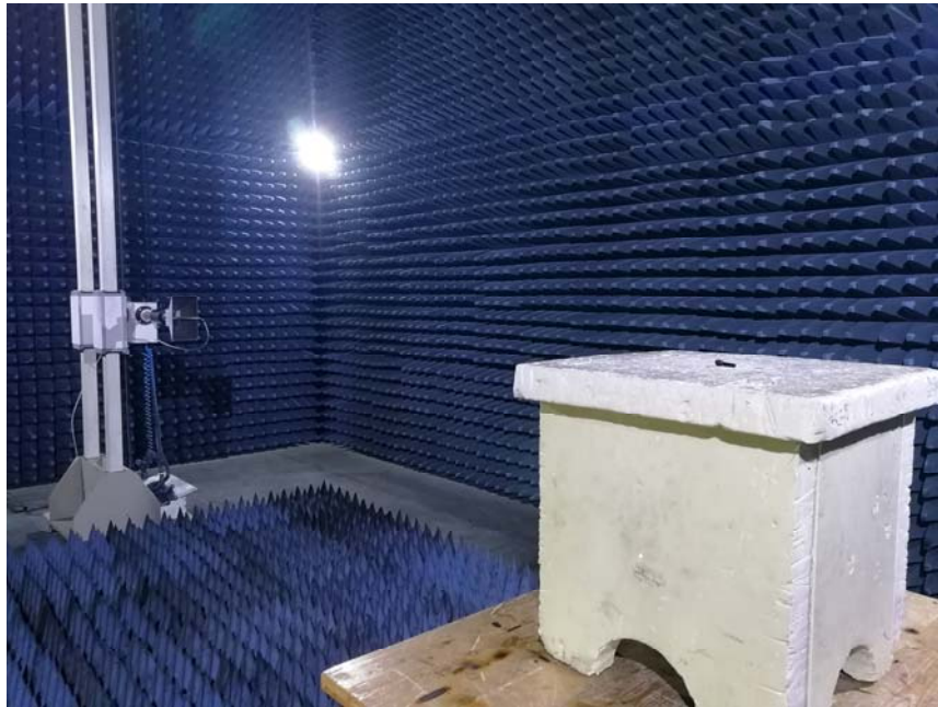
Photograph of set-up for conducted Emission
