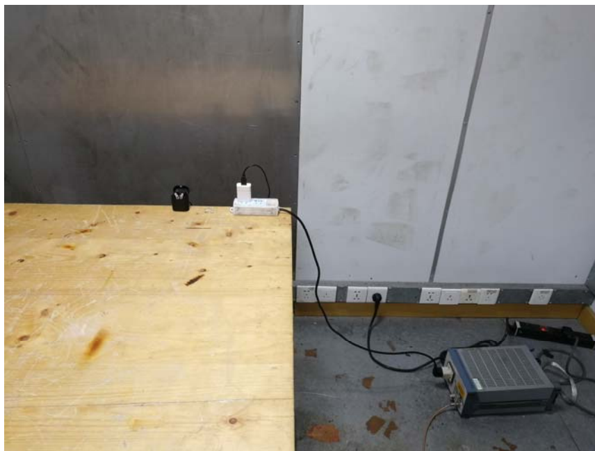
Photograph of set-up for conducted Emission
