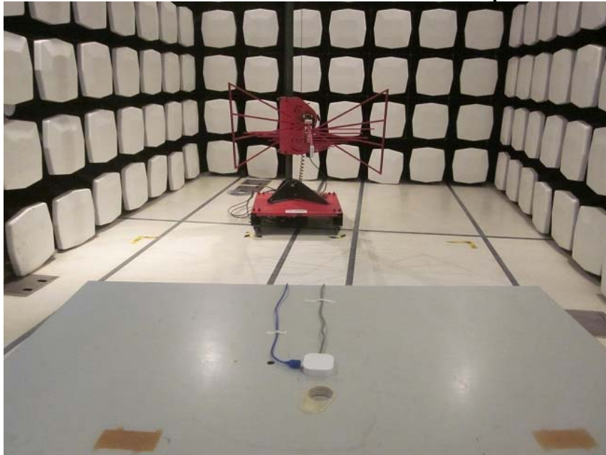
Measurement of Radiated Emission Test Set Up
