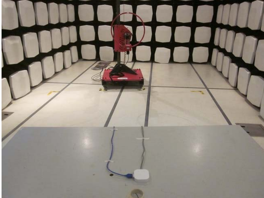
Measurement of Radiated Emission Test Set Up
