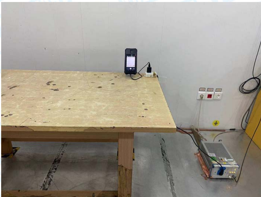
Photo of Setup for Conducted Emission
