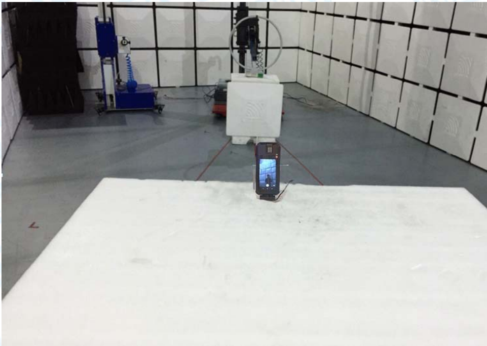
Photo of Setup for Conducted Emission
