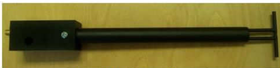
Figure 1 – MVG COMOSAR Validation Dipole
