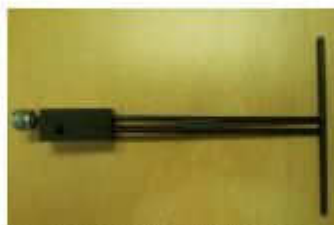
Figure 1 – MVG COMOSAR Validation Dipole
