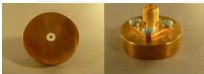
Figure 1 – MVG LIMESAR Dielectric Probe
