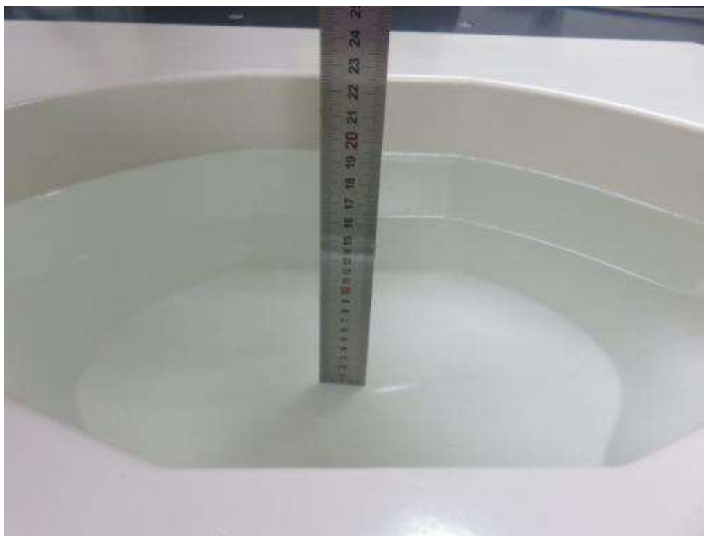
Photograph of the depth in the Body Phantom (750MHz, 16.1cm depth)
