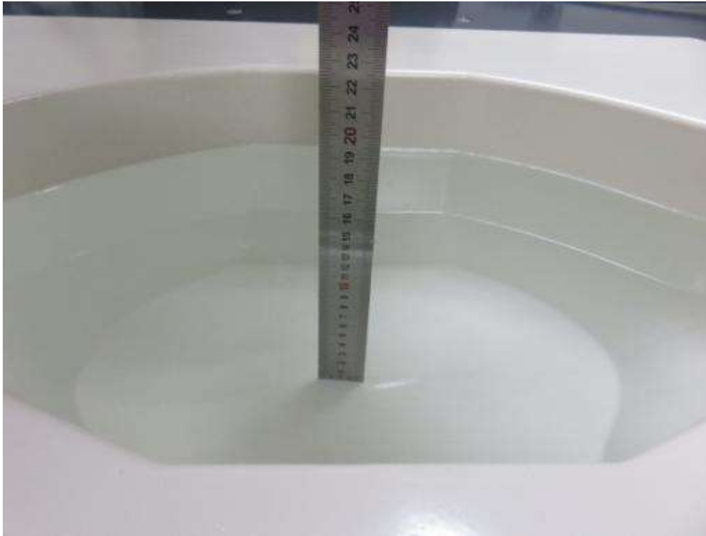
Photograph of the depth in the Body Phantom (5200MHz, 16.3cm depth)
