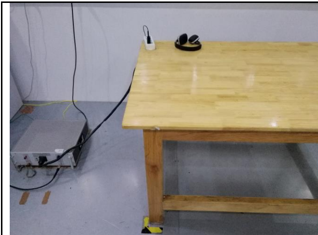
Conducted Emissions Test Setup Front View
