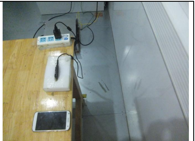
Conducted Emissions Test Setup Side View
