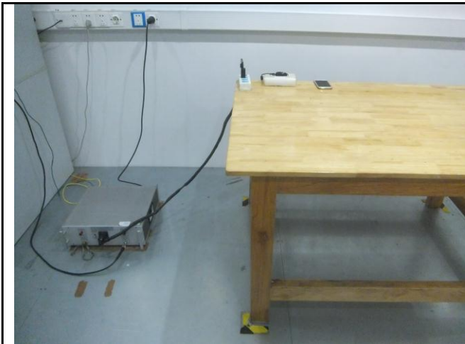
Conducted Emissions Test Setup Front View
