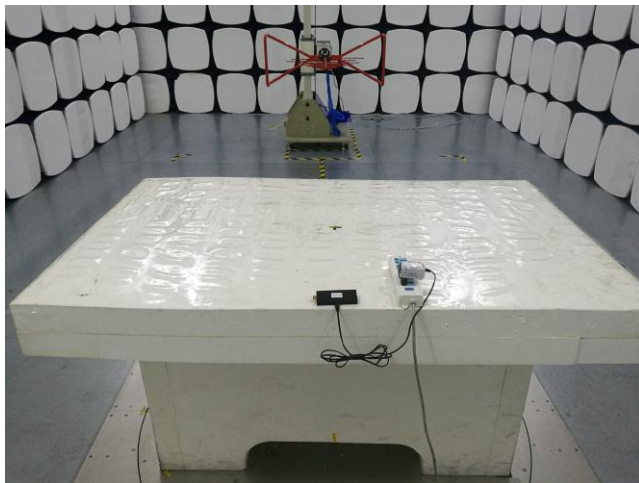
Conducted Emissions Test Setup Front View
