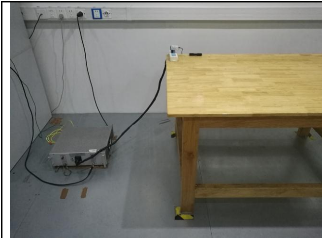
Conducted Emissions Test Setup Front View
