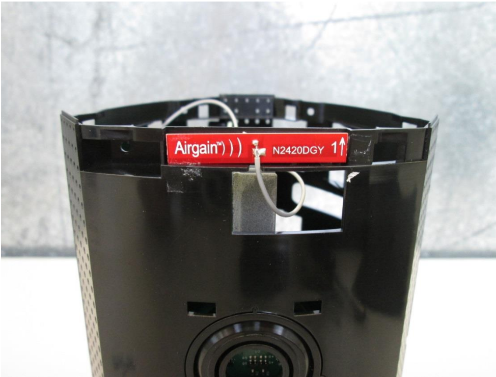
Photo A2-7: Placement of Antenna #1
