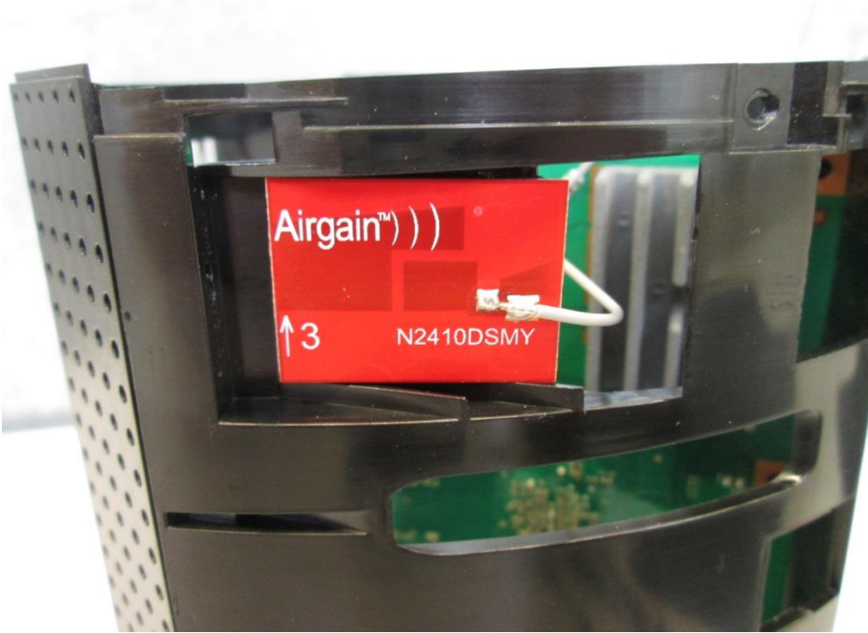
Photo A2-9: Placement of Antenna #3
