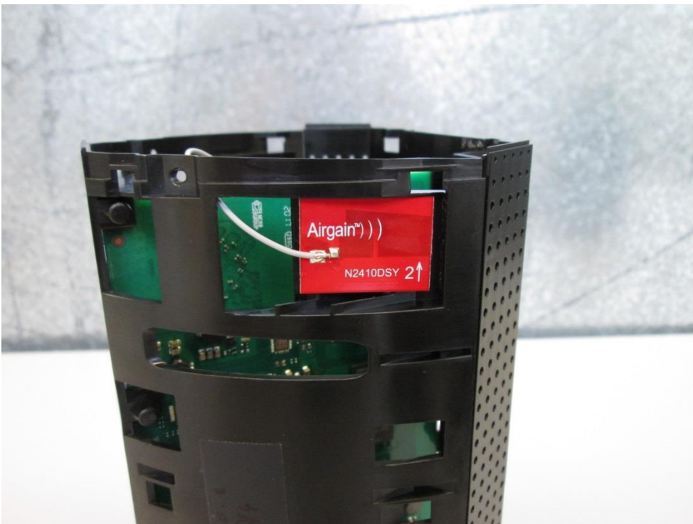
Photo A2-8: Placement of Antenna #2
