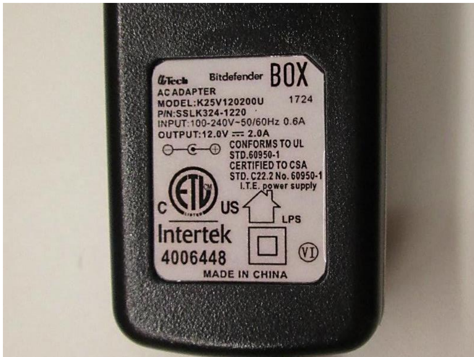
Photo A4-2: Label of AC/DC Adaptor
