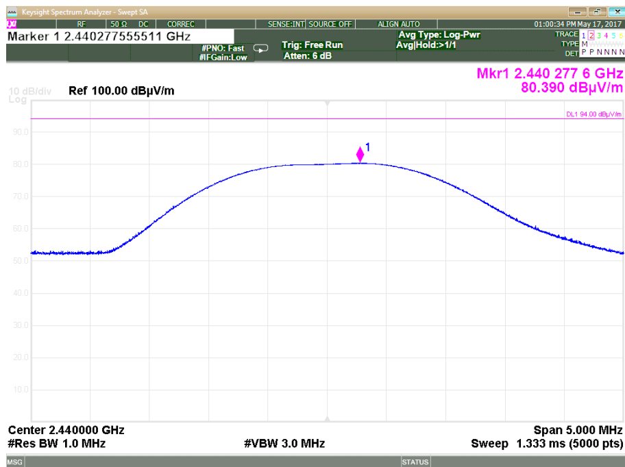
Plot 3.2.4: Radiated Emissions test, Horizontal Polarization, Tx Modulated, Field strength of fundamental, Fc -2440
