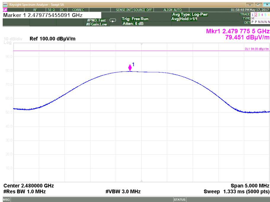
Plot 3.2.6: Radiated Emissions test, Horizontal Polarization, Tx Modulated, Field strength of fundamental, Fc -2480
