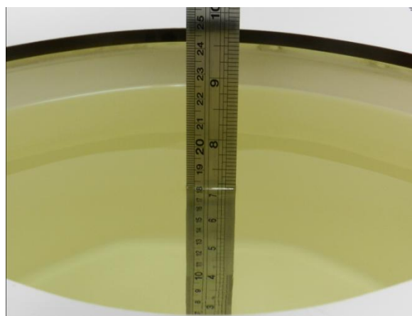
Fig 10.2 Photo of Liquid Height for Body SAR
