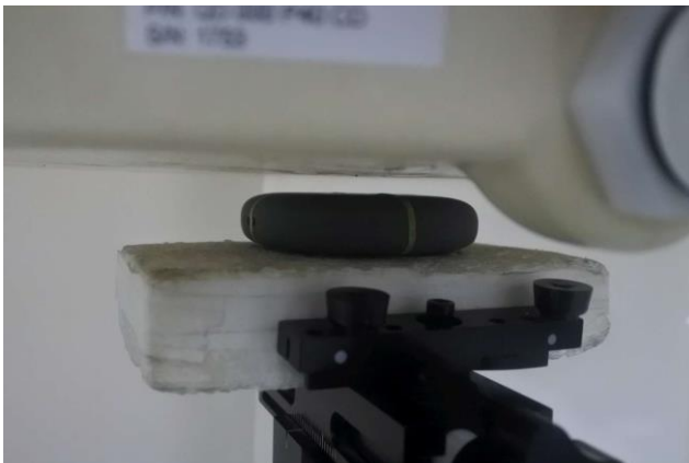
In front of face, Test Separation 5 mm
