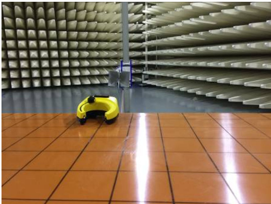
Spurious Radiated Emissions Test setup (1GHz~25GHz)
