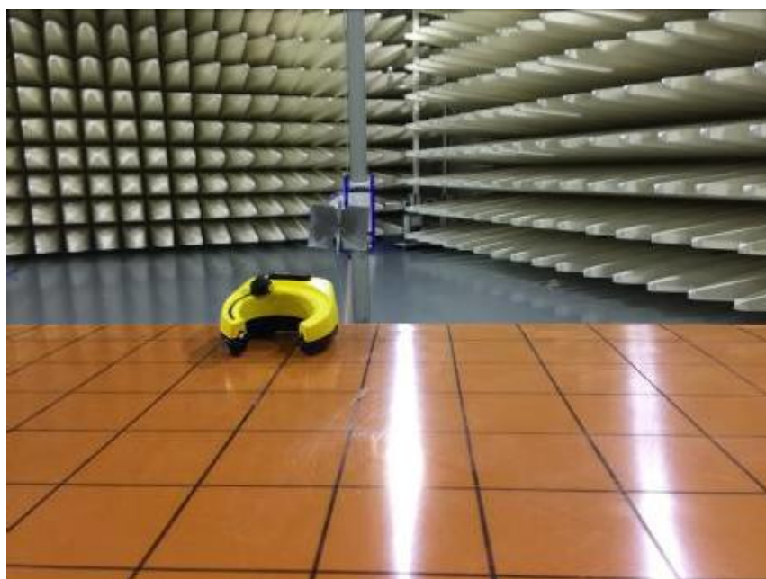
Radiated Spurious Emissions Test setup
