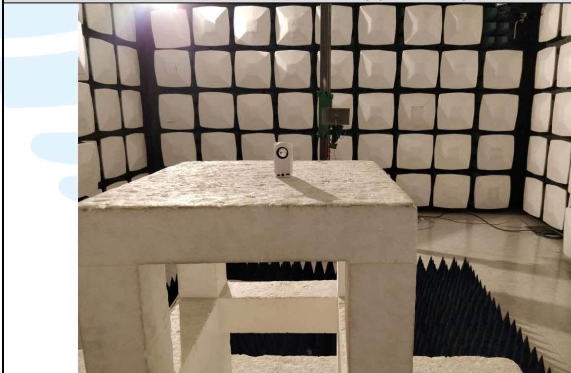
Radiated emission Test Setup (Above 1 GHz)
