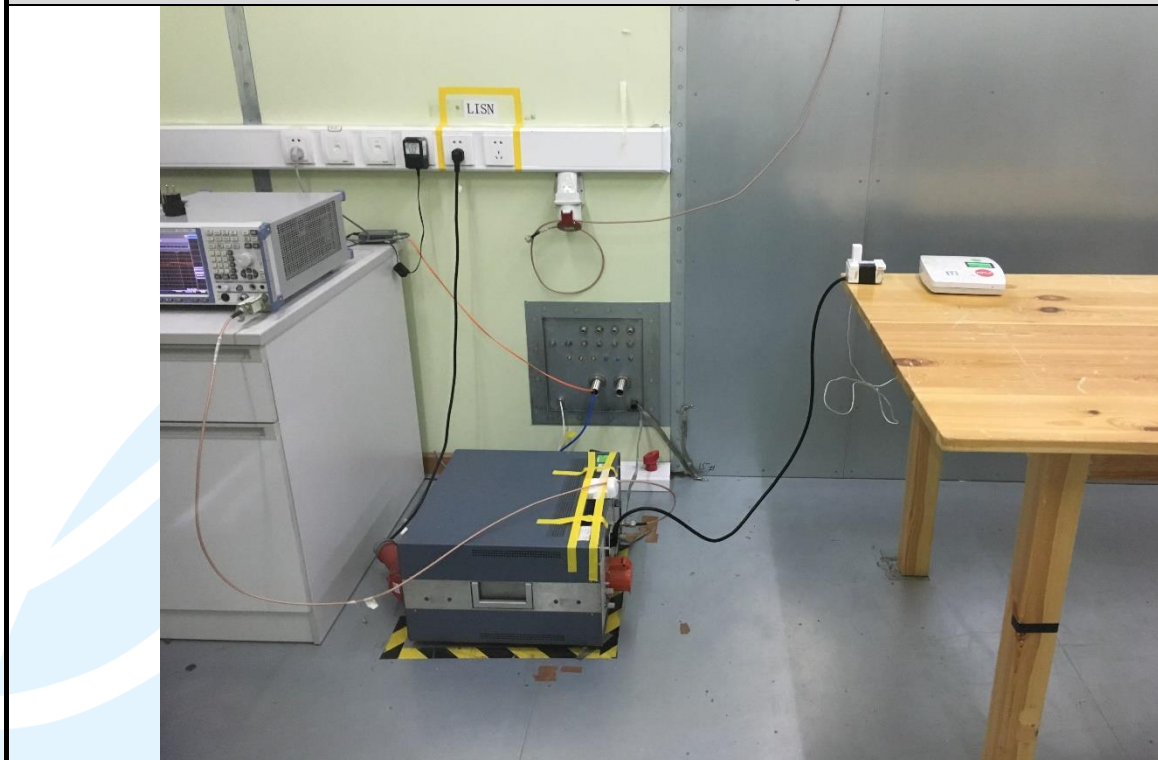
Conducted Emission Test Setup - Mode 1
