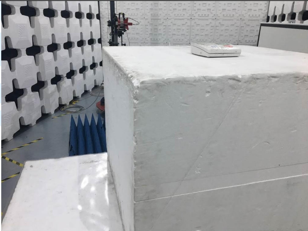
Radiated emission Test Setup (Above 1 GHz) - Mode 3
