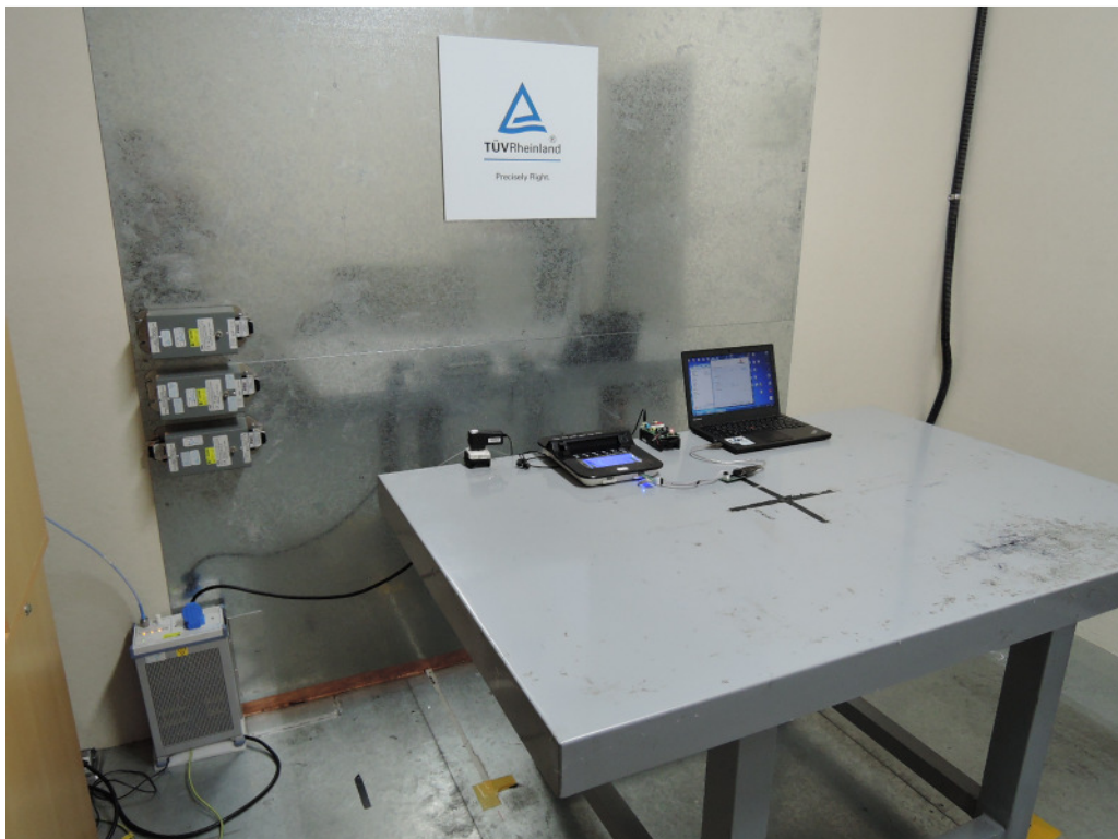
Photograph 7: Set-up for for Mains Conducted testing Front
