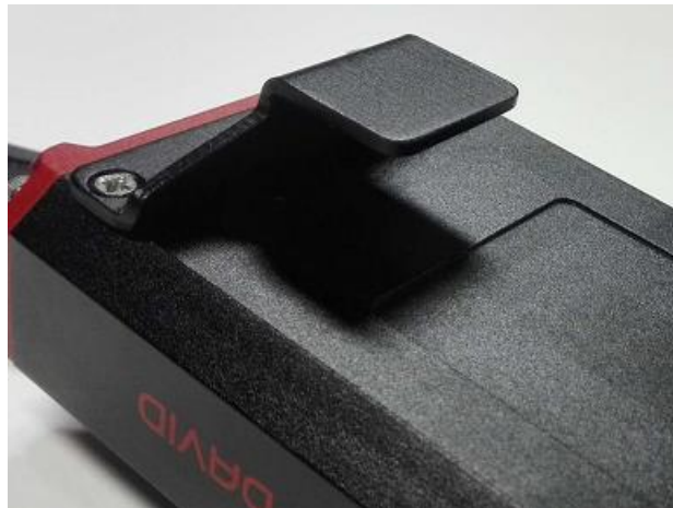
Figure 37 David GNSS receiver installation hook
