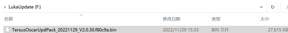
Figure 2.22 The FW is placed in the LUKAUpdate removable disk
