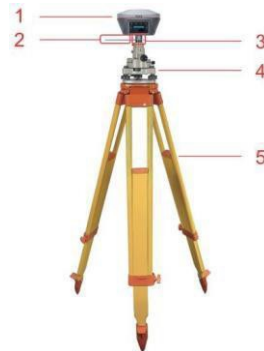
Figure 4.1 Oscar Trek as a base - network mode
