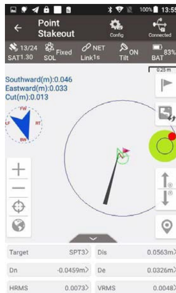
Figure 4.21 Point stakeout when tilt compensation is on
