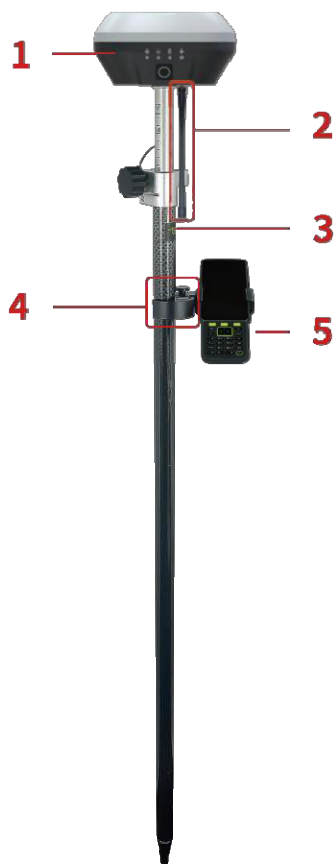
Figure 1.2 TS21 as a Rover – Internal Radio
