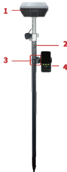
Figure 1.1 TS20 as a Rover – Network Mode
