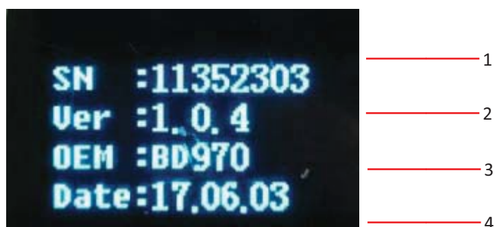
Figure 2-9 Receiver status information
