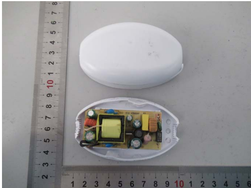
EUT – Adapter Mainboard Top View
