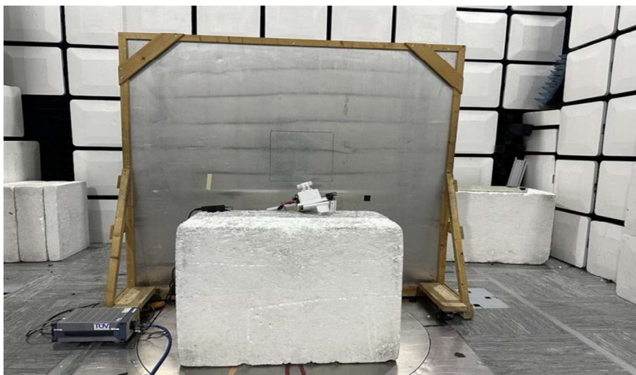
Figure 38 – AC Power Line Conducted Emissions Face On
