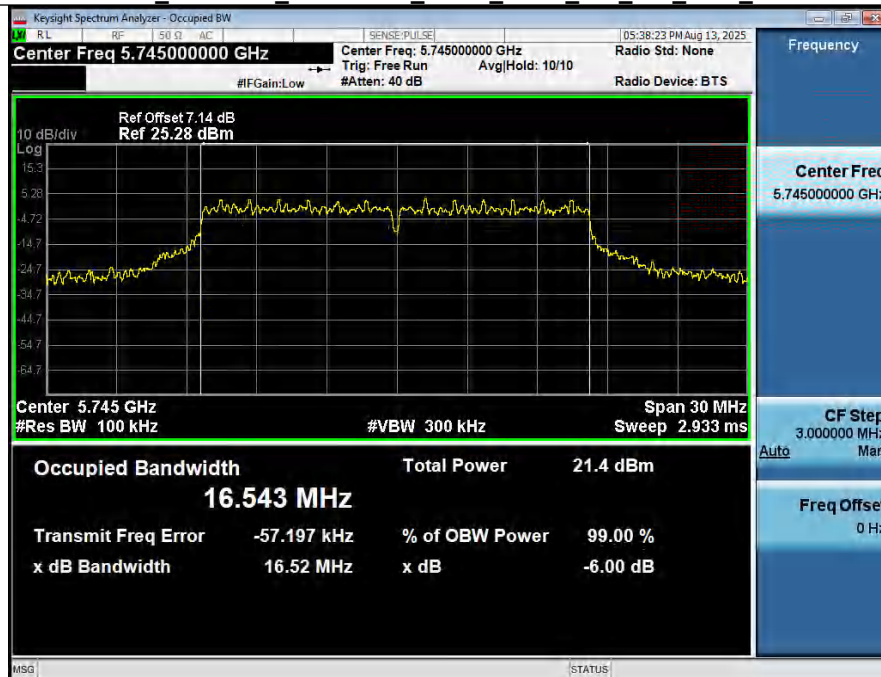
-6dB Emission Bandwidth NVNT_ANT2_802_11a_5745_20M
