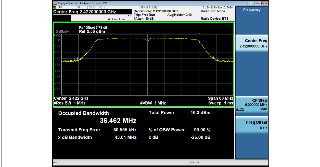
99% Occupied Bandwidth NVNT_ANT2_802_11n(HT40)_2422
