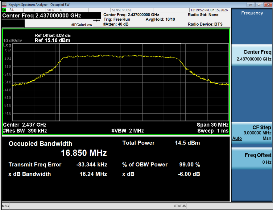
-6dB Bandwidth NVNT ANT2 802 11g 2437
