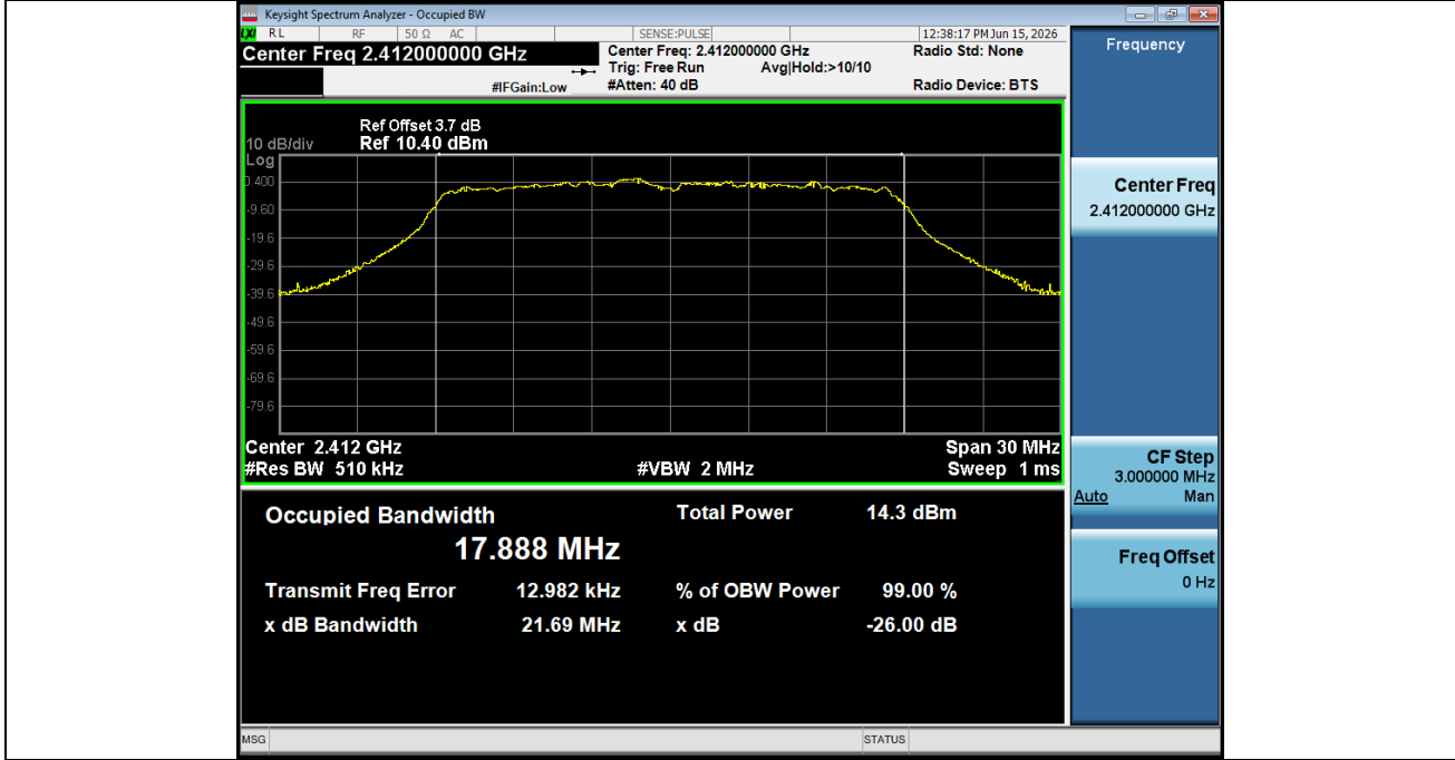
99% Occupied Bandwidth NVNT_ANT2_802_11n(HT20)_2412
