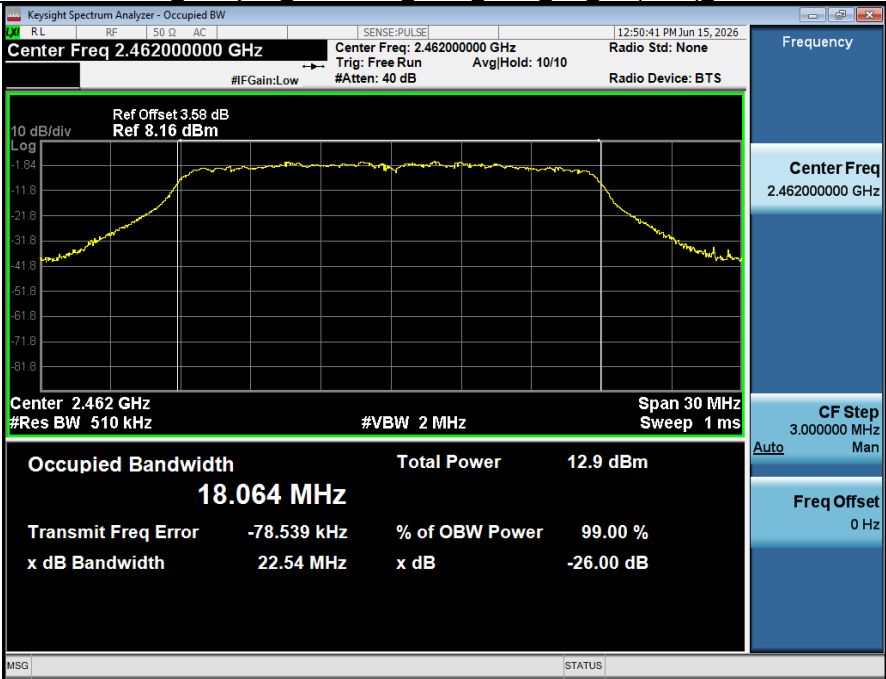
99% Occupied Bandwidth NVNT_ANT2_802_11n(HT20)_2462
