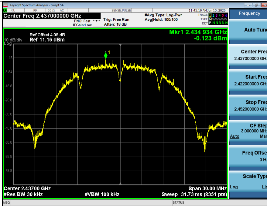
Power Spectral Density NVNT ANT2 802 11b 2437
