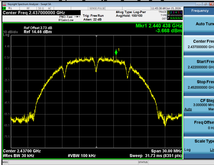
Power Spectral Density NVNT ANT2 802 11b 2437
