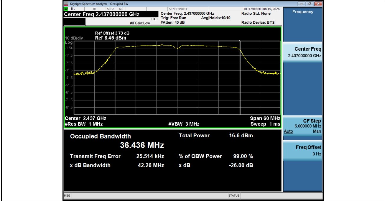
99% Occupied Bandwidth NVNT_ANT2_802_11n(HT40)_2437
