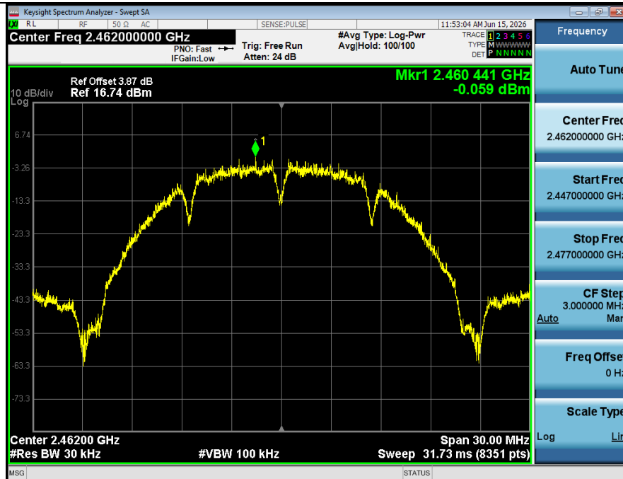
Power Spectral Density NVNT ANT2 802 11b 2462
