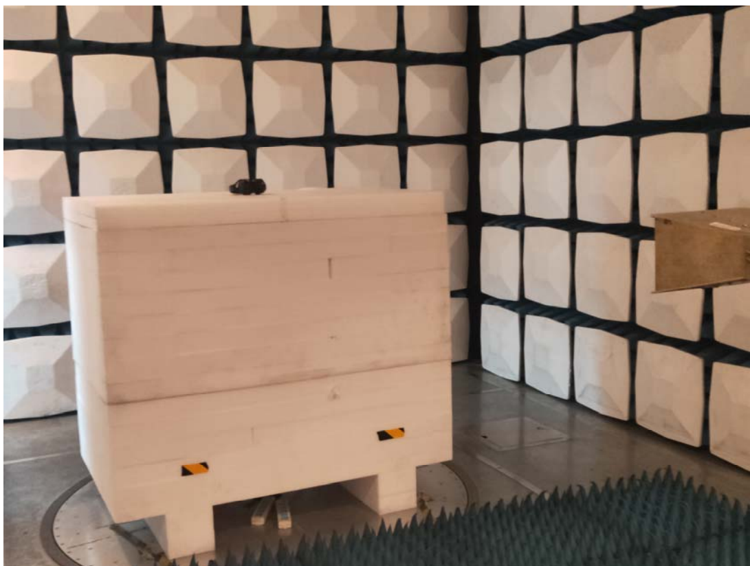
Radiated Emission Above 1GHz View
