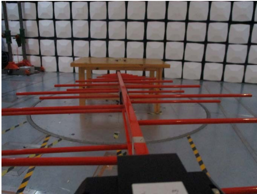
Radiated Emission View (Below 1GHz)
