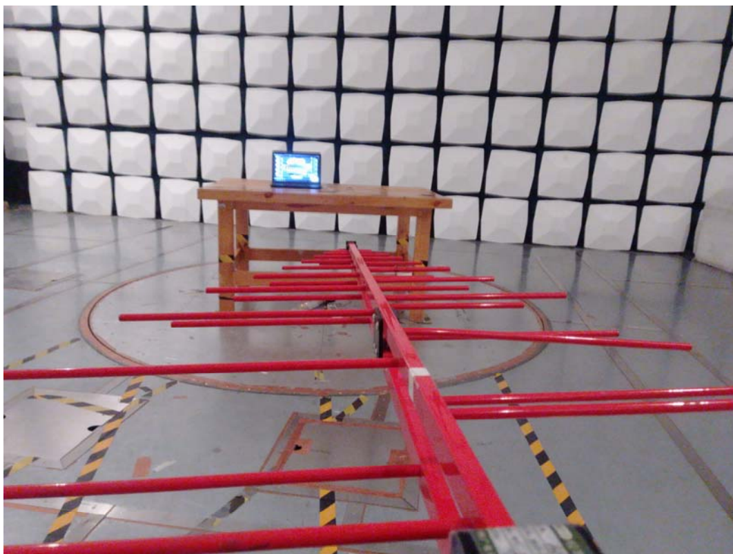
Radiated Emission Above 1GHz View
