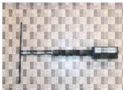
Figure 1 – Satimo COMOSAR Validation Dipole
